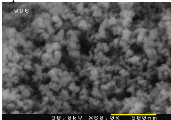
Figure 2. SEM images of prepared magnetite nanoparticles
