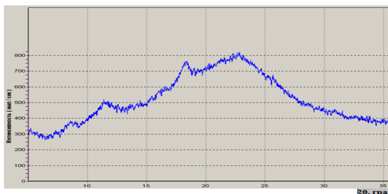
Figure 2. The XRD pattern of chitosan film in salt form. MMhtz = 420 kDa, SD = 0.8 . Composition spinning solution: Shtz = 2 wt%, Suk = 2 wt%, CH_2O = 96 wt%. Film air-dry
