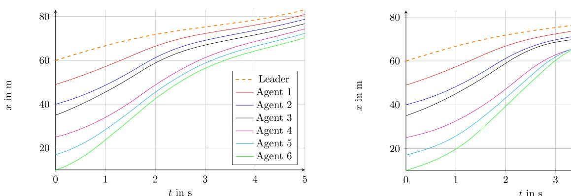
Time-delays and packet dropouts degrade the performance and can cause collisions! Moreover, large initial spacing errors can not be handled.
