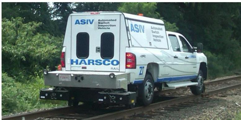
Abbildung 34 Automated Switch Inspection Vehicle [13]
