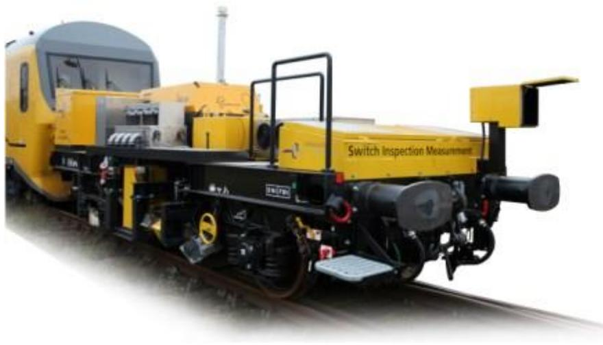
Abbildung 27 Switch inspection and measurement system [77]
