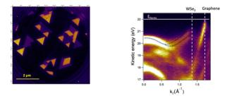
Figure 1. left: Dark field LEEM image of WSe<sub>2</sub> triangular islands on graphene obtained by chemical vapor deposition. Right:  $\mu$ -ARPES measurements of the band dispersion from the  $\Gamma$  to the K point for the heterostructure formed by monolayer WSe<sub>2</sub> supported on monolayer graphene.
