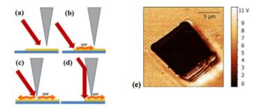
Figure 1 (a)-(d) Different contributions to s-SNOM pattern: (a) incident s-SNOM laser (b) edge excited SPPs (c) tip-launched SPPs (d) tip reflected edge excited SPPs (e) Resulting s-SNOM image (second harmonic of the AFM vibration) of a window in an Au layer on ITO substrate reveals the superposition of the different contributions.
