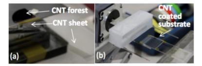
Figure 1. a) Realization of CNT sheets: b) Substrate coated with layer of aligned CNTs
