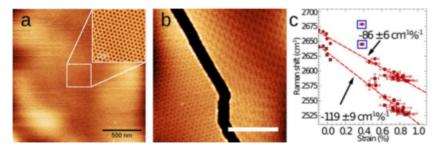
Fig. 1. a) AFM images of moiré patterns on the surface of epitaxially grown graphene on hBN, (inset) high resolution image of the central region of the main image. b) AFM image of a crack in a graphene monolayer exhibiting regular and highly anisotropic moiré patterns. Scale bar 175 nm. c) Raman shift of graphene 2D peak positions as a function of strain, determined by spatial correlation of local moiré periodicity with Raman peak position.
