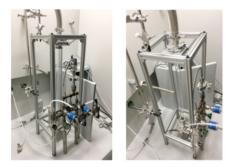
Figure. The fluidized bed reactor (FBR) configuration for coating nanoparticles using ALD.
