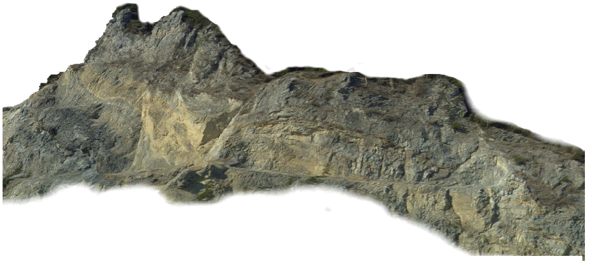
Fig. 1 Metric 3D image of a quarry. The image size is about 92 Megapixels. The 3D model consists of about 1,000,000 points. The image was recorded from a distance of 700 m using the JointMetriX3D panorama scanner.
