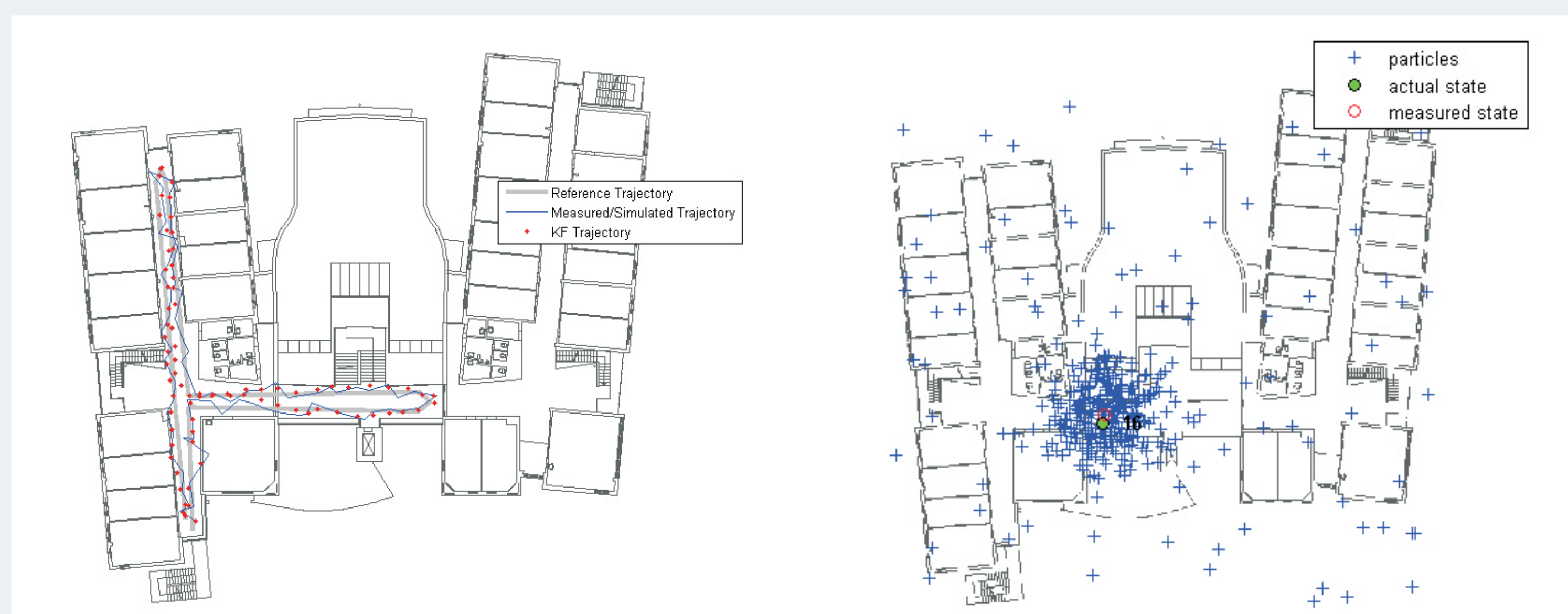
Figure 3: Kalman Filter (left graph) compared to the Particle Filter (right graph)
