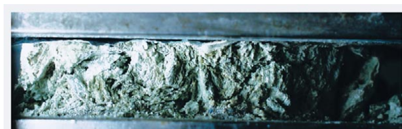
Deformations of weak faulted phyllite Brittle cataclastic flow- interlayer shear
