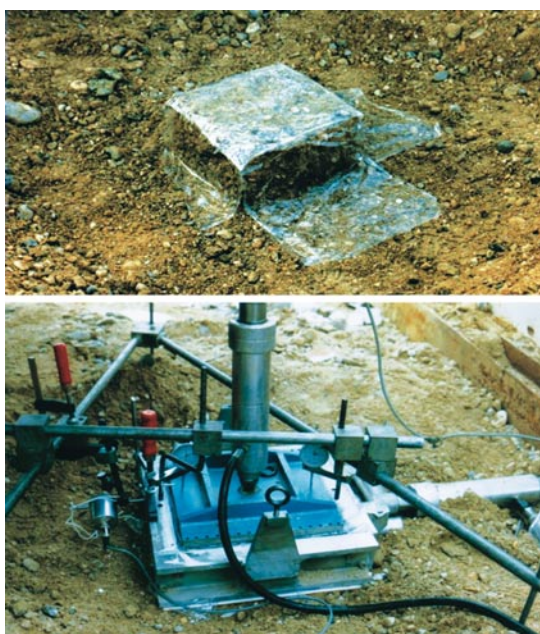
Fig. 2 In-situ direct shear test.
