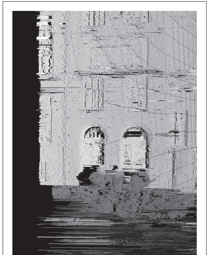
Figure 11. Point cloud from image triplet of the scene in Figure 8, processed on PC with one GPU in 2 seconds.
