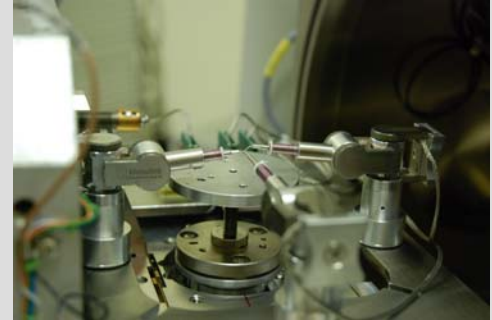
Fig. 1: Micromanipulator installed in a FEI Quanta 200 (photograph taken by Kleindiek)
