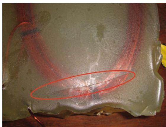
Figure 4.13: Crack caused by thermal stress
