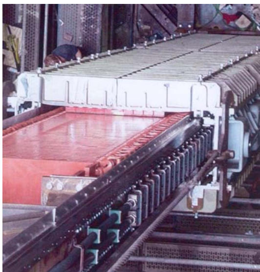
Figure 3.13: The AWS' linear generator during assembly (Source: AWS)
