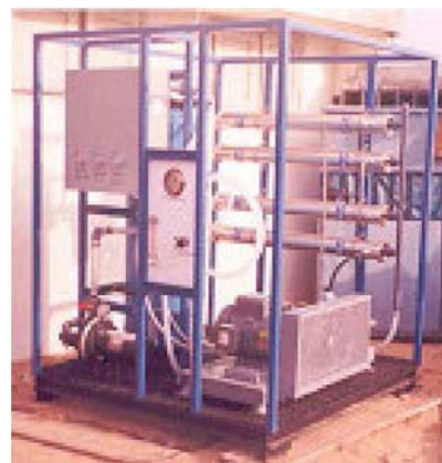
Figure 3.4: Desalination unit (from [42])
