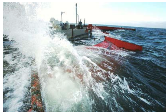
Figure 3.27: Wave Dragon in action (Source: Wave Dragon ApS)
