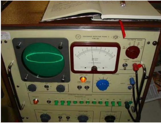
Figure 4.28: Out-Dated Discharge Detector
