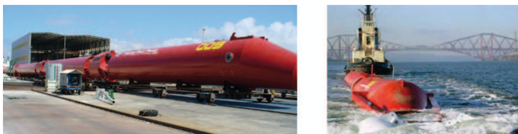
Figure 3.16: Pelamis wave energy converter: One of the units that have been sold to Portugal (left); a prototype (right) on it's way for open sea tests in Edinburgh (Source: Ocean Power Delivery Limited)
