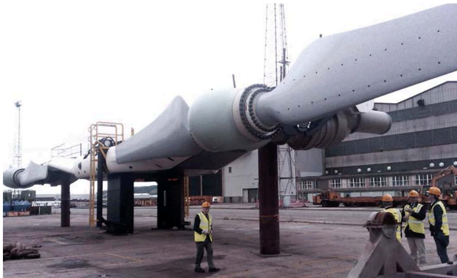
Figure 3.37: A SeaGen rotor assembly before installation (from Wikipedia.org)
