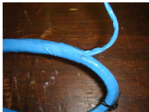
Figure 4.9: The connection-wire egression needs special caring
