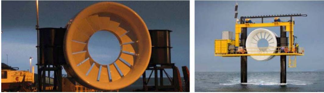
Figure 3.39: Open-Center Turbine before installation (left), mounted prototype Installation at Orkney, Scotland (right, both pictures from OpenHydro)
