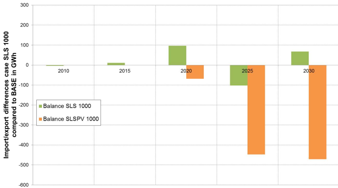
Figure 38: Changes in import export compared to BASE case for SLS 1000 MW and SLSPV 1,000 MW
