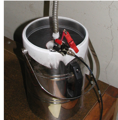
Figure 5: Cable model with open-cell foam as insulation medium (left) and test vessel (right)
