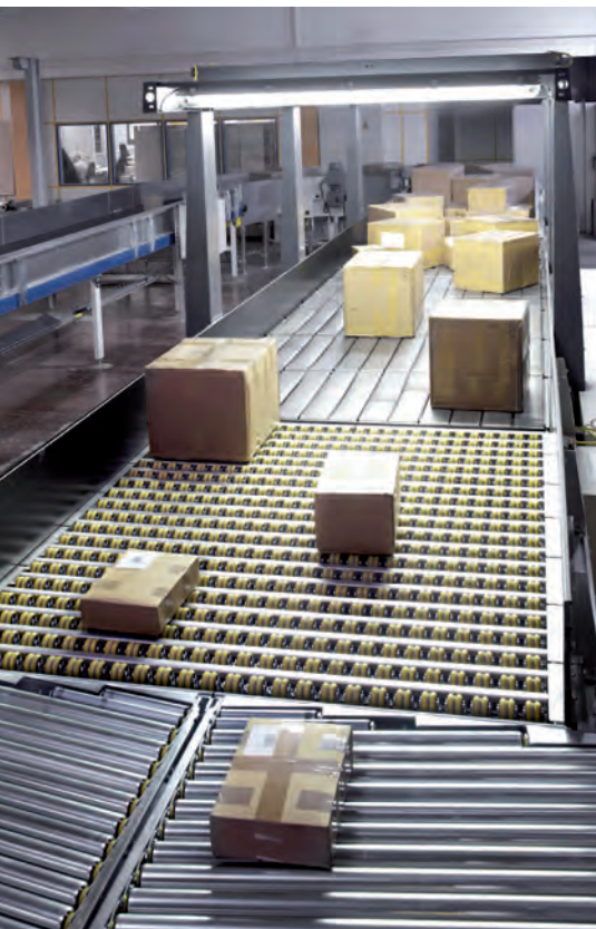
02 Adjustable drive segments in active isolation systems, such as the Vision Singulator by Siemens, correct the position and direction of each individual item
