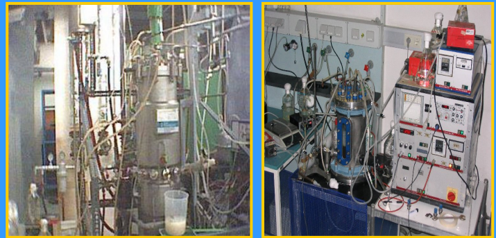
Figure 4: MBR 42 liter bioreactor (biosynthesis of copolyester; left picture) and L 1523 Bioengineering bioreactor (biosynthesis of terpolyester; right picture)
