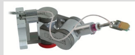
Fig. 3: Micromanipulator with force measurement plug-in tool (photograph taken by Kleindiek)
