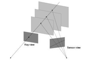
Figure 8: Plane sweeping principle. The homography between the façade's reference plane and the sensor view varies for different depths.
