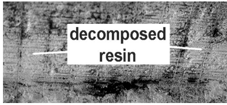
Fig. 5. Decomposed epoxy resin on the surface of copper strands.
