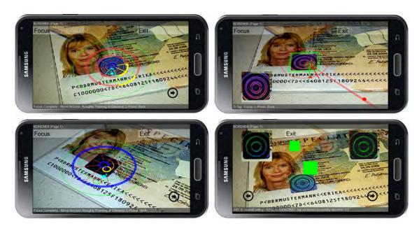
Figure 5.13: User interfaces for hologram verification: Constrained navigation (top-left), alignment (top-right) and hybrid user interfaces (bottom-left) are designed, implemented and evaluated within a user study. They allow to reliably capture image data suitable for automatic verification. Results are presented to the user in a summary (bottom-right).
