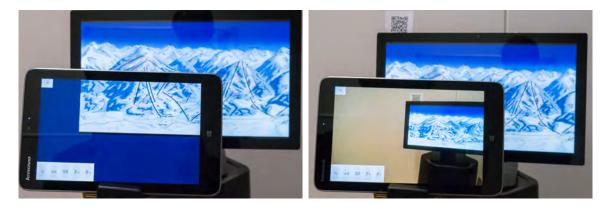
**Figure 6.2:** (left) Simultaneous 3D head tracking and *NFT* enable user perspective magic lenses for situated display content. (right) Device perspective rendering usually found in handheld Augmented Reality devices.
