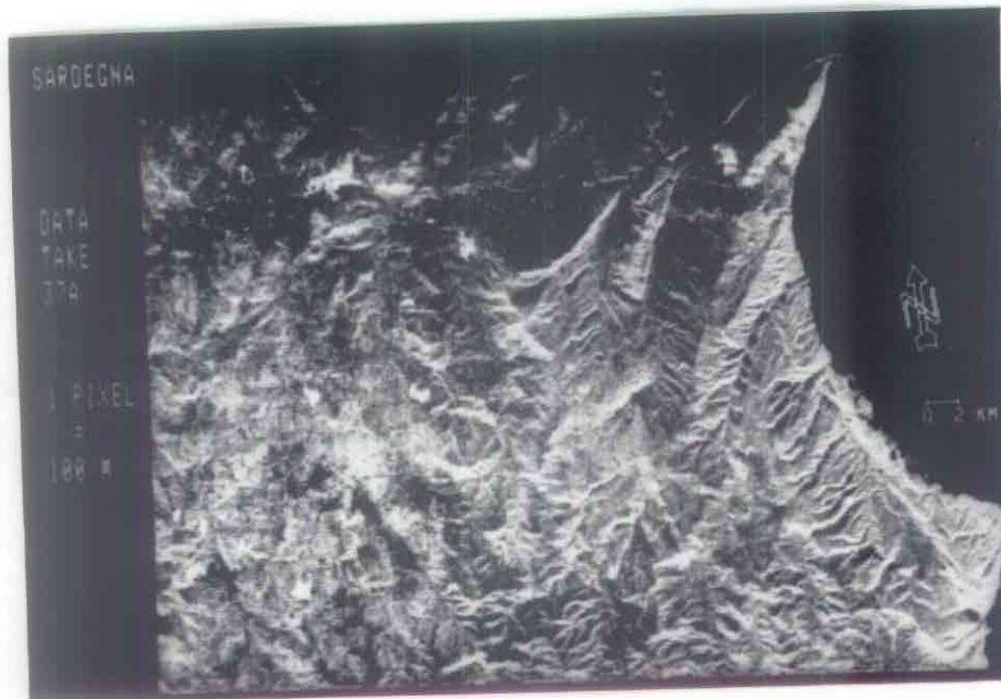
FIGURE 17a: Digitized SIR-A image, Data Take 37A. Averaged by a factor of 9.
