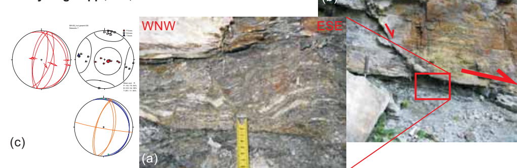
Figure 4: Quarry Ungerlipp (Marhof). (a) A major normal fault parallel to the foliation cuts through the quarry, again cataclastic sheared Plattengneis forms the fault core. Note tilting towards W of the foliation in the shear zone. (b) Listric normal fault terminates in foliation parallel shear zone, note synthetic splays and tensile fractures in the hanging wall. (blue great circle = foliation, green cross = stretching lineation, orange great circle = discontinuity with unclear genesis)
