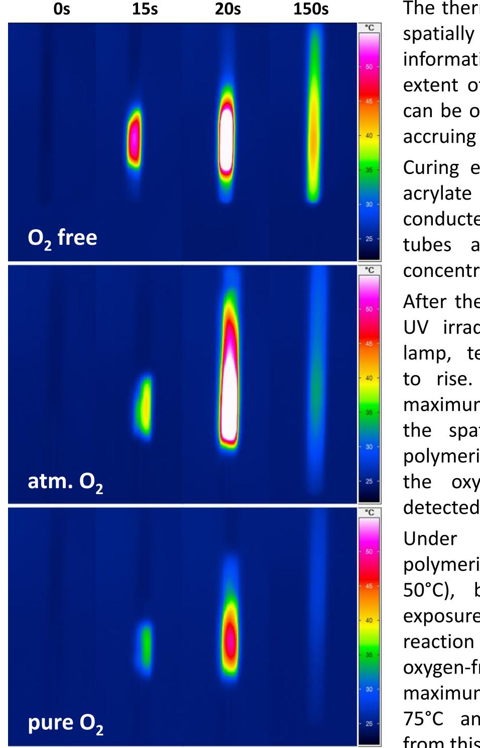
The thermal camera provides spatially resolved curing information. Here, the spatial extent of the polymerization can be observed through the accruing reaction heat.
