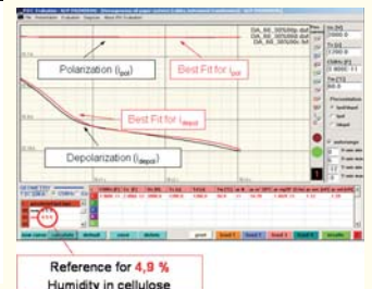
Figure 6: Determination of water content with PDC analysis
