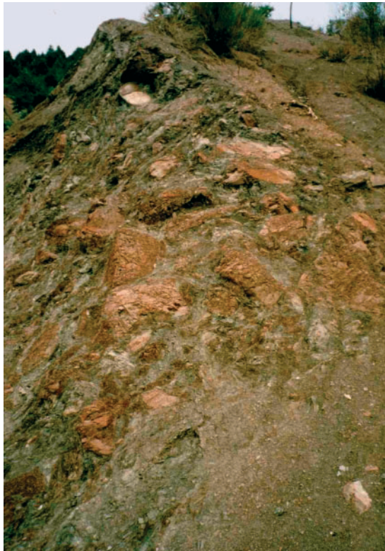
Fig. 7 Bimrock developed along a thrust fault in "Red Flysch". Blocks of sandstone varying in size and shape are surrounded by clayey gouge.
