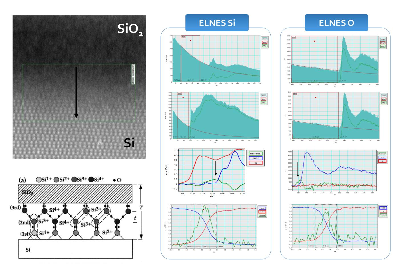
**Fig.2:** HR STEM HAADF of transition region, schematic of transition [1] (left) Analysis of ELNES signal of Si and O (right)
