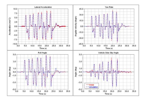
Fig. 7 Comparison simulation-measurement: Multiple lane change.
