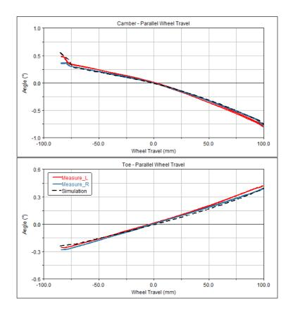
Fig. 6 Camber and toe angles during parallel wheel travel from simulations and measurements.
