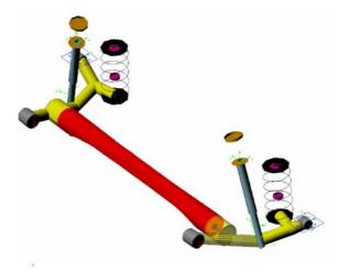
Fig.2 Rear suspension model.
