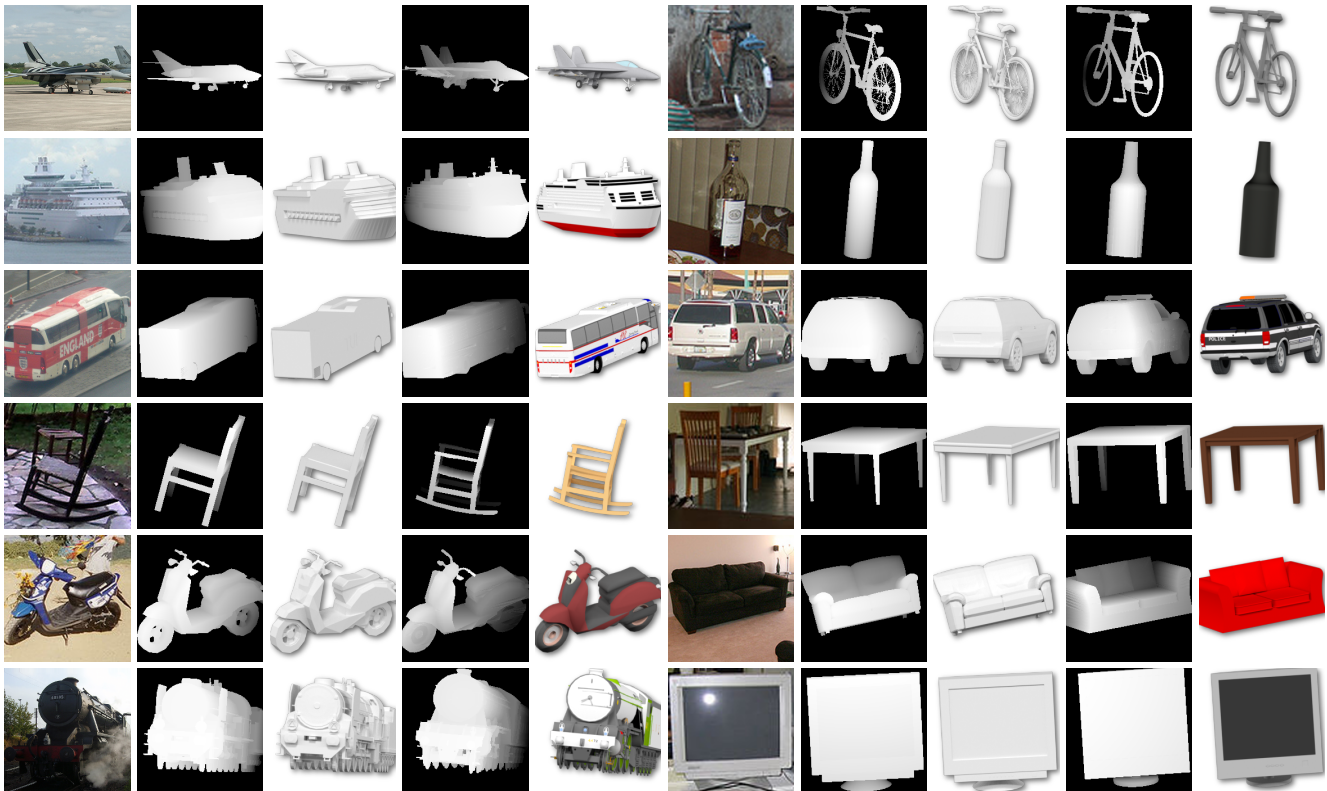
Figure 4: Qualitative results for 3D pose estimation and 3D model retrieval from ShapeNet given images from Pascal3D+ for all twelve categories. For each category, we show: the query RGB image; the depth image and RGB rendering of the ground truth 3D model from Pascal3D+ under the ground truth pose from Pascal3D+; the depth image and RGB rendering of our retrieved 3D model from ShapeNet under our predicted pose. We provide more results in the supplementary material.
