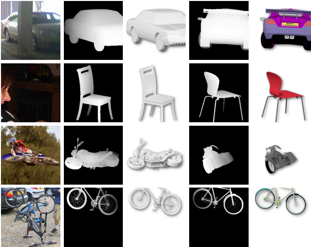
Figure 10: 3D pose estimation fails in difficult situations (same image arrangement as in Fig. 7). We observe that heavy occlusions (first row), bad illumination conditions (second row) and difficult object poses (third and fourth row), which are far from the poses seen during training, result in incorrect pose predictions. In the last row, we see that not even the annotated ground truth pose is correct.
