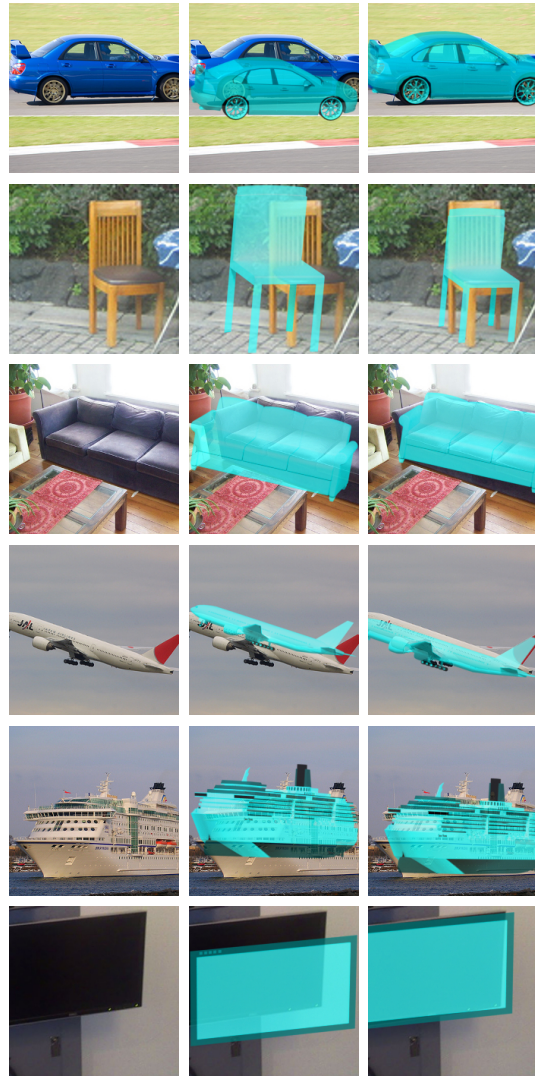
Figure 8: We use our predicted 6-DoF pose and 3-DoF dimensions to refine the alignment between the object and a rendering. Left: A detected object, which is not centered on the image window. Middle: A rendering which just uses our predicted 3-DoF rotation. Right: A rendering which uses our predicted 6-DoF pose and 3-DoF dimensions.
