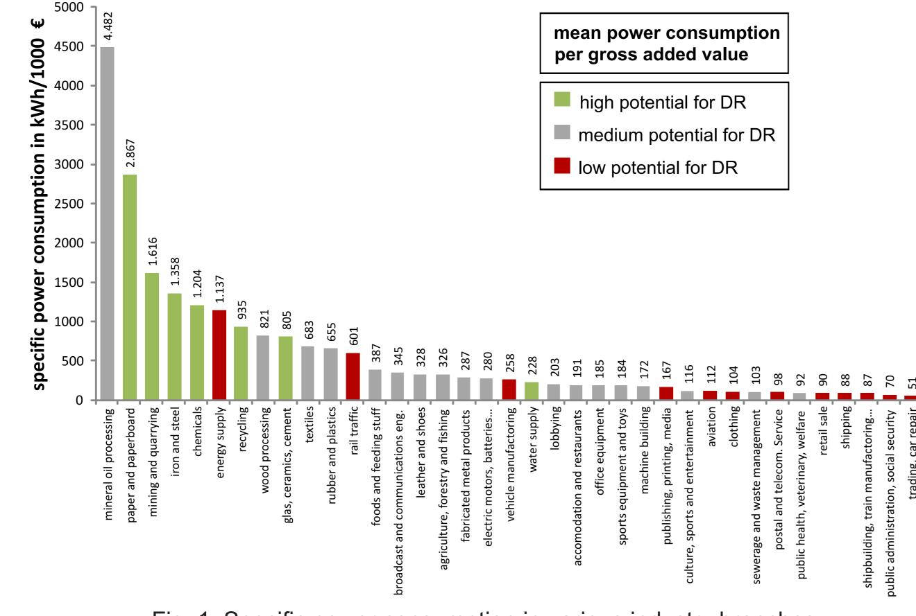
Fig. 1: Specific power consumption in various industry branches
