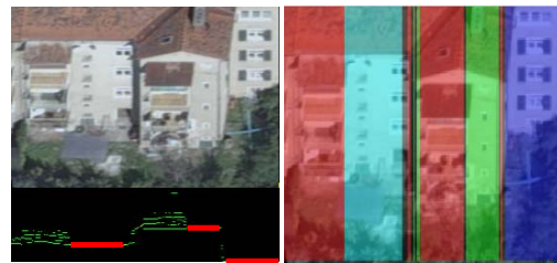
Figure 7: Plane detection for a complex facade; (a) key-view of a facade and projection in xy-plane (red lines are strongly weighted (>66% of points lie in this plane)); (b) determined major façade planes (segmented areas with balconies are marked in red)
