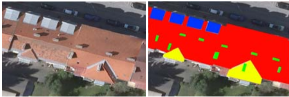
Figure 10: Segmentation of a roofscape into different roof categories (red: major planes; yellow: minor planes; green: chimneys; blue: dormer windows). [Source: Detail of the Graz test dataset]
