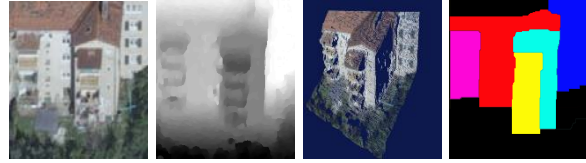
Figure 6: Reconstructed building façades using plane sweeping. (a) key view of façade (b) raw 3D point cloud (c) 3D point cloud overlaid with RGB information (d) segmentation of that point cloud into façade areas belonging to specific vertical planes
