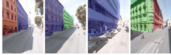
Figure 1: Four examples of automatically segmented street side images into individual building facades. Use is being made of overlapping street-side images. In this example, the camera is pointed forward (from Recky M. et al., 2011).
