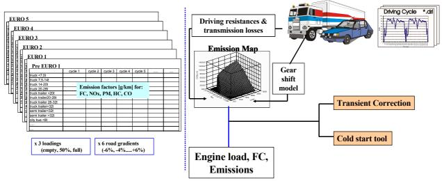
Figure 1: Emission factors to be modelled and diagram of the model PHEM from TU-Graz
