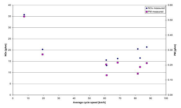
Figure 26: NO<sub>x</sub> and PM -emissions measured for a EURO 2 HDV on the chassis dynamometer
