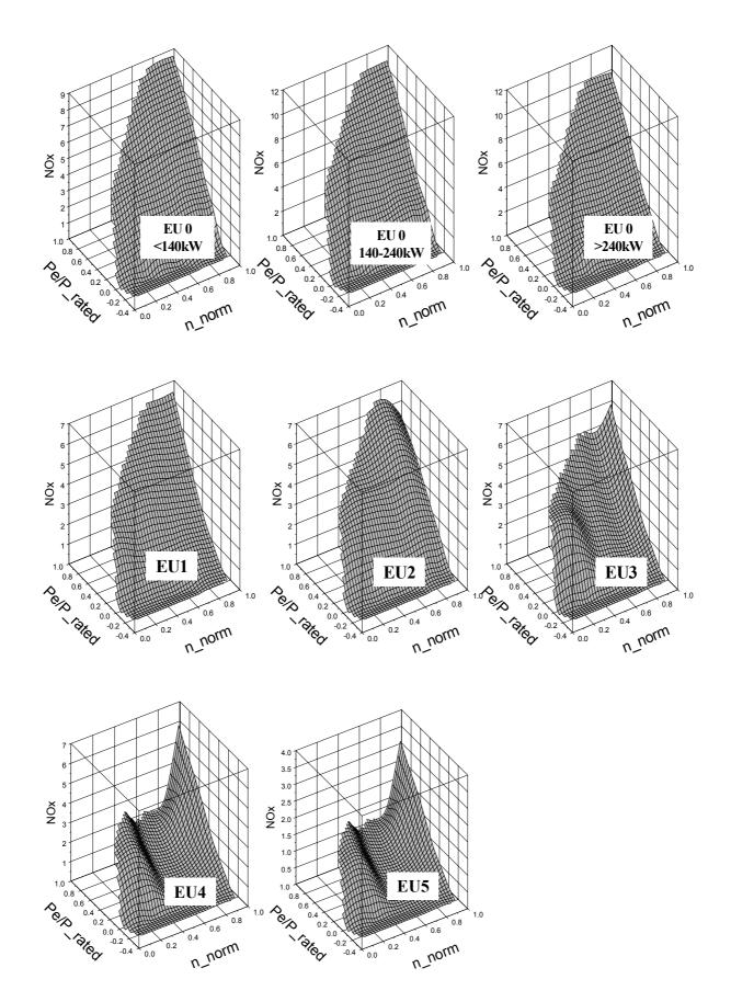
Figure 79: NO<sub>x</sub>-emission maps for the average technology classes (standardised map formats, values in (g/h)/kW <sub>Rated Power</sub>
