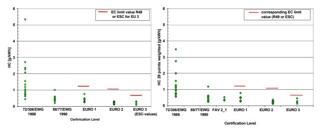
Figure 14: HC-emissions in the type approval tests (left) and in the weighted 29-point map (right).
