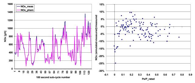
**Figure 55:** Difference between measured and simulated NO<sub>x</sub>-emissions for the average of all EURO 2 engines in all 100 second sub cycles of all transient tests plotted over the cycle time (left) and over the average engine power demand of the sub cycle (right)
