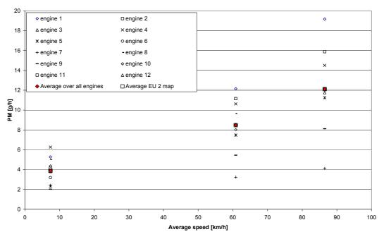
**Figure 40:** Simulated particulate emissions for a truck-configuration using all single engine emission maps available for EURO 2 compared to the simulation with the average EURO 2 engine map.
