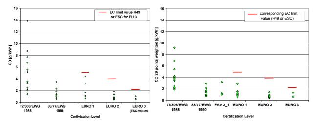
Figure 13: CO-emissions in the type approval tests (left) and in the weighted 29-point map (right).
