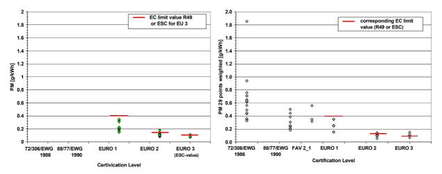
Figure 15: Particle-emissions in the type approval tests (left) and in the weighted 29-point map (right).
