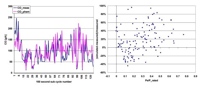
**Figure 57:** Difference between measured and simulated CO-emissions for the average of all EURO 2 engines in all 100 second sub cycles of all transient tests plotted over the cycle time (left) and over the average engine power demand of the sub cycle (right)
