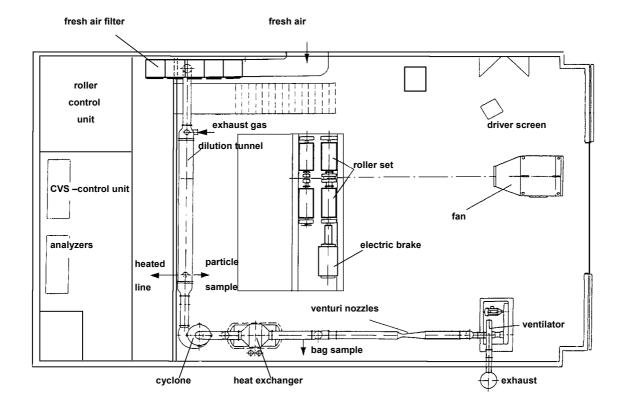
The chassis dynamometer and the main parts of the CVS system are given in the following figure.
