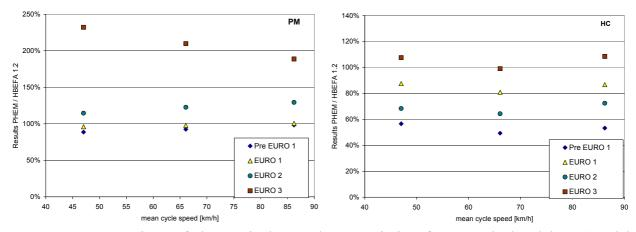
**Figure 99:** Comparison of the particulate and HC emission factors calculated here (model PHEM) with the emission factors from the Handbook Emission Factors (HBEFA 1.2) for three driving cycles with 0% road gradient, 50% loaded solo truck 14-20t
