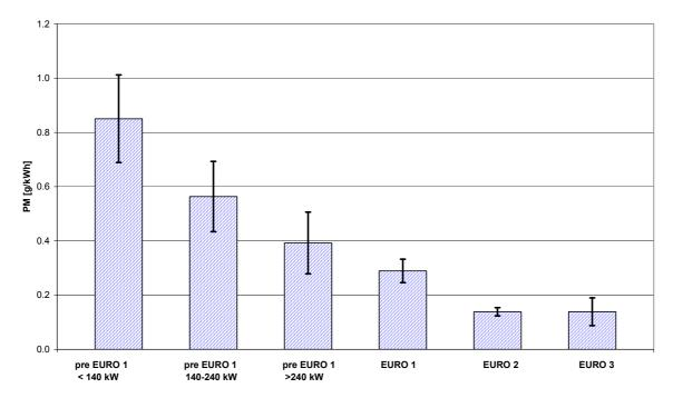
Figure 47: Average emission value in the standardised 32 point engine map and 95% confidence interval of these value for the engine categories.
