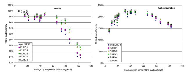
**Figure 94:** Ratio of average cycle speed and fuel consumption for 100% loaded and empty HDV in the category "semi trailer and truck trailer 34-40t" for +/-2% road gradient
