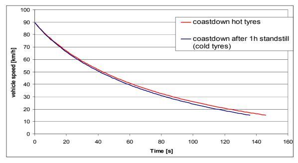
Figure 61: Measured vehicle speed at the coast down tests on the chassis dynamometer with cold and hot tyres
