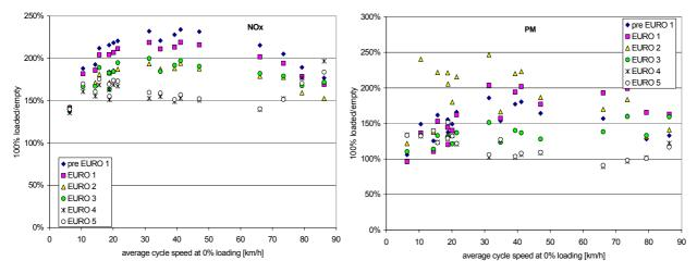
Figure 96: Ratio of NOx and PM emissions for 100% loaded and empty HDV in the category "semi trailer and truck trailer 34-40t" for +/-2% road gradient
