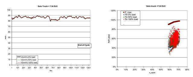
Figure 84: Cycle 1020 (Highway standard, 0% gradient) simulated with a solo truck < 7.5t, EURO 3 (cycle= left, engine load = right)
