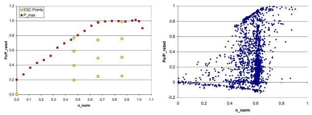
Figure 70: European Stationary Cycle (ESC) and European Transient Cycle (ETC) in the engine map, example for an EURO 3 engine
