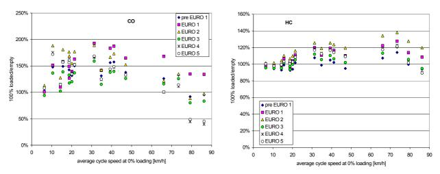
Figure 97: Ratio of CO and HC emissions for 100% loaded and empty HDV in the category "semi trailer and truck trailer 34-40t" for +/-2% road gradient
