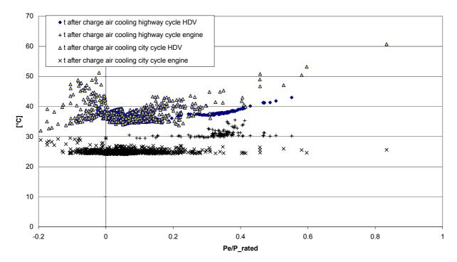
Figure 58: intake air temperatures in a slow city cycle and a fast highway cycle (HDV=measured on chassis dynamometer; engine = interpolated from engine test bed measurement)
