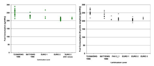
Figure 11: Fuel consumption in the type approval tests (left) and in the weighted 29-point map (right).
