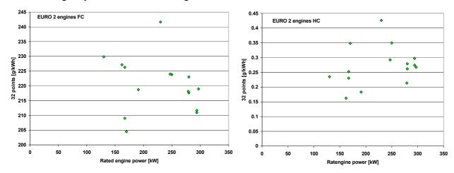
Figure 36: Average fuel consumption and HC-emission values in the standard engine maps over the rated engine power for EURO 2 engines
