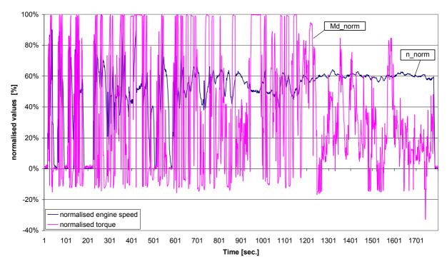
Figure 16: European Transient test Cycle (ETC)
