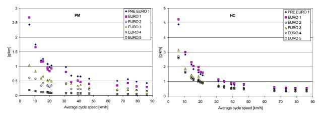
Figure 90: Simulated particulate and HC-emission factors for truck trailers and semi trailers 34 to 40 tons, 50% loaded, 0% road gradient
