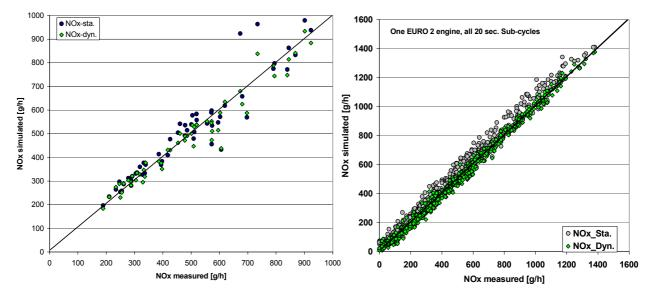
**Figure 45:** NO<sub>x</sub>-emissions simulated with and without transient correction functions compared to the measured values for all engines in all available transient tests (left) and for one EURO 2 engine in all 20-second sub-cycles (right)
