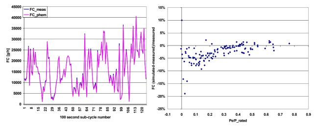
**Figure 54:** Difference between measured and simulated FC for the average of all EURO 2 engines in all 100 second sub cycles of all transient tests plotted over the cycle time (left) and over the average engine power demand of the sub cycle (right)
