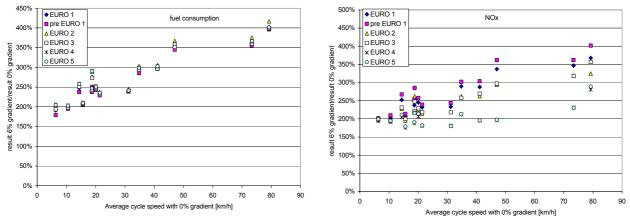
Figure 92: Comparison of fuel consumption and NOx emissions on a flat road to 6% road gradient
