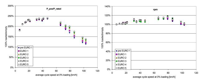
Figure 95: Ratio of average positive engine power needed and average engine speeds for 100% loaded and empty HDV in the category "semi trailer and truck trailer 34-40t" for +/- 2% road gradient
