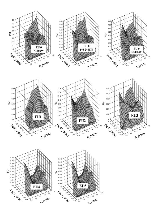
Figure 80: Particulate matter-emission maps for the average technology classes (standardised map formats, values in (g/h)/kW Rated Power
