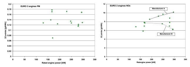
**Figure 35:** Average PM- and NO<sub>x</sub>-emission values in the standard engine maps over the rated engine power for EURO 2 engines
