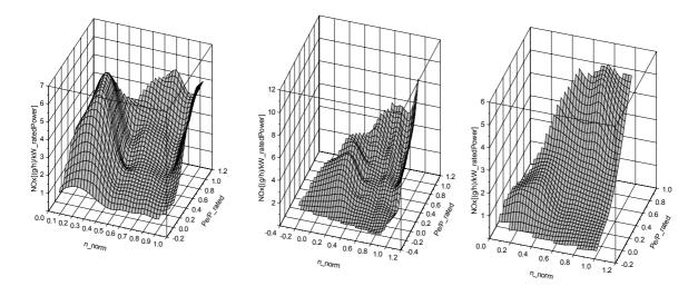
Figure 10: Steady-state NO<sub>x</sub>-engine emission map for three Euro 3 engines
