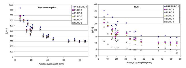
Figure 89: Simulated fuel consumption and NO<sub>x</sub>-emission factors for truck trailers and semi trailers 34 to 40 tons, 50% loaded, 0% road gradient
