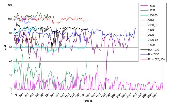
Figure 25: Driving cycles for the measurements on the chassis dynamometer.
