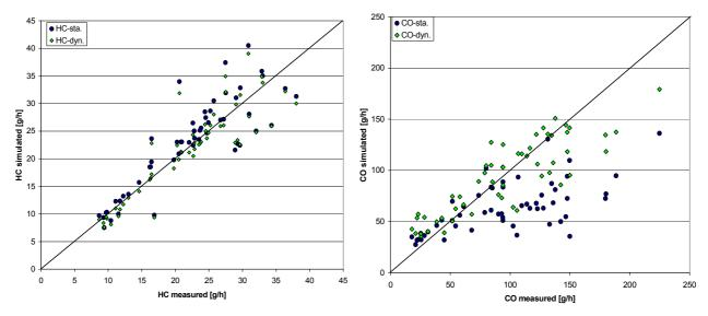
For CO similar improvements can bee seen as for particulates while the accuracy for HC emissions is also without transient correction functions astonishing good (Figure 46).
