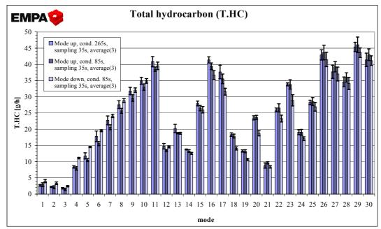
Figure 7: THC emissions at three different measurement modes of the ARTEMIS steady state test
