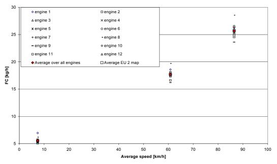
Figure 39: Simulated fuel consumption of a truck-configuration using the single engine emission maps available for EURO 2 compared to the simulation with the average EURO 2 engine map.
