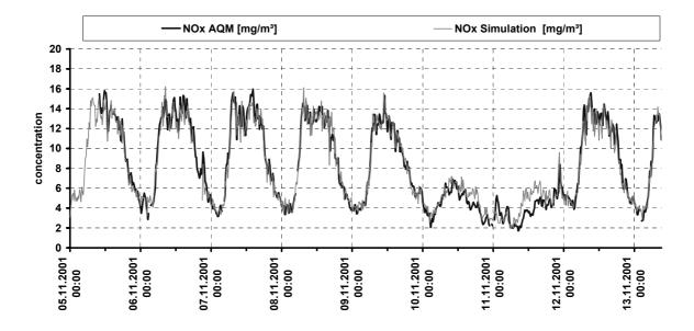
Figure 104: Comparison between measured and calculated NO<sub>x</sub> concentrations for a period of 8 days
