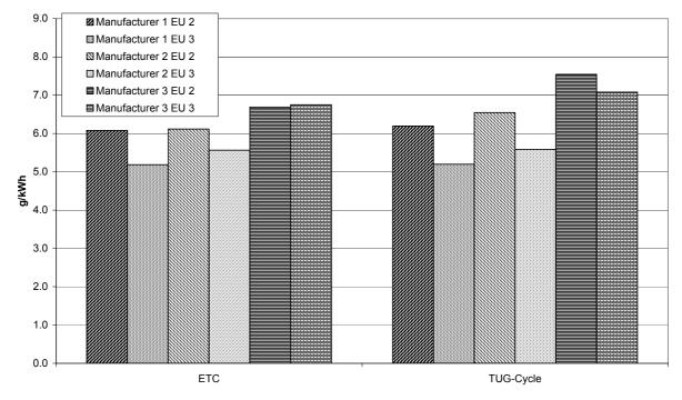
Figure 21: Measured NO<sub>x</sub>-emissions for three EURO 3 engines and for the predecessor Euro 2 engines from different manufacturers in two different transient cycles
