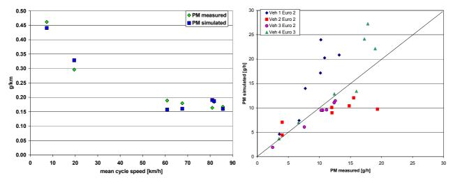
Figure 68: Comparison of particulate emissions measured on the chassis dynamometer versus the simulated values for the average of all HDV (left) and for all single HDV (right)
