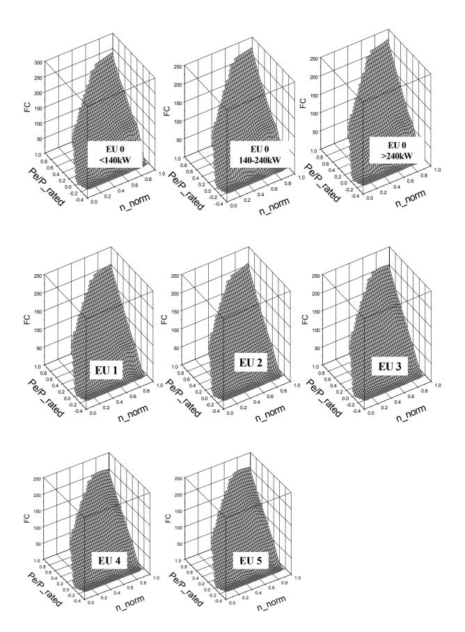
Figure 78: Fuel consumption maps for the average technology classes (standardised map formats, values in (g/h)/kW Rated Power
