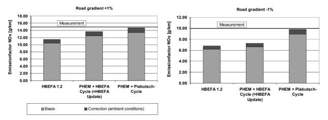
Figure 103: Comparison of emission factors gained by tunnel measurements and by calculation with HBEFA 1.2 and the new model PHEM
