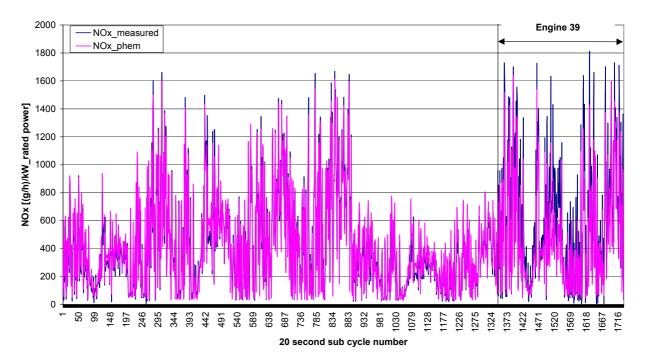
**Figure 49:** Measured and simulated NO<sub>x</sub> emissions in the 20-second sub cycles for all transient tests of all EURO 3 engines.
