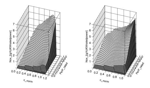
Figure 8: Typical steady-state NO<sub>x</sub>-engine emission map for Euro 1 engines
