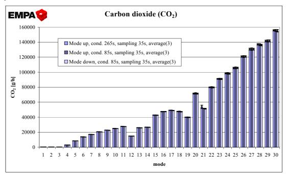
Figure 4: CO<sub>2</sub> emissions at three different measurement modes of the ARTEMIS steady state test
