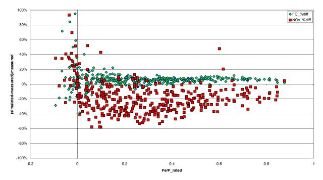
**Figure 50:** Difference between measured fuel consumption and NO<sub>x</sub> emissions to the simulated values in the 20-second sub cycles of all transient tests for engine 39.
