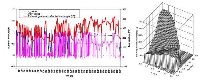
Figure 71: Measured exhaust gas temperatures at an EURO 3 engine in a real world test cycle (TNO 7.5 kW/ton cycle) and resulting engine temperature map.
