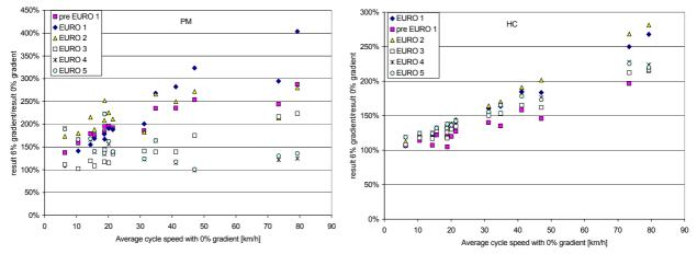
Figure 93: Comparison of particulate and HC emissions on a flat road to 6% road gradient
