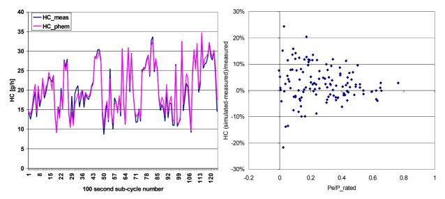
**Figure 56:** Difference between measured and simulated HC-emissions for the average of all EURO 2 engines in all 100 second sub cycles of all transient tests plotted over the cycle time (left) and over the average engine power demand of the sub cycle (right)
