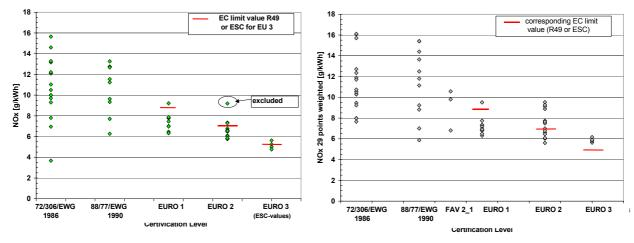
Figure 12: NO<sub>x</sub>-emissions in the type approval tests (left) and in the weighted 29-point map (right).
