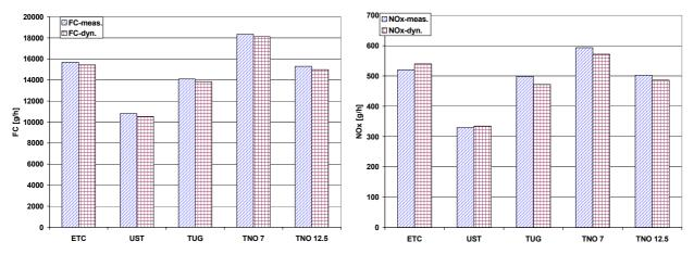
Figure 52: Average measured fuel consumption and NO<sub>x</sub> emissions vs. simulation results (-dyn.) for all EURO 2 engines.
