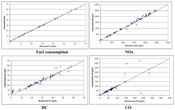
Figure 33: Measured steady state emission values and results of the interpolation from the standard 32 point engine map format
