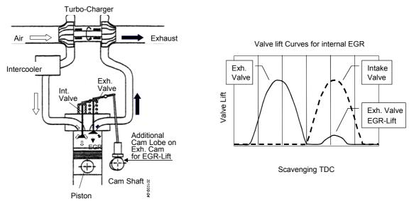
Figure 76: Internal EGR (Source: Hino Motors Limited)
