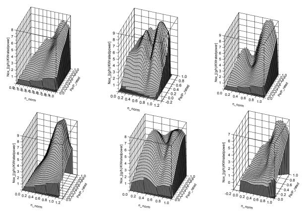
Figure 9: Steady-state NO<sub>x</sub>-engine emission map for six different Euro 2 engines
