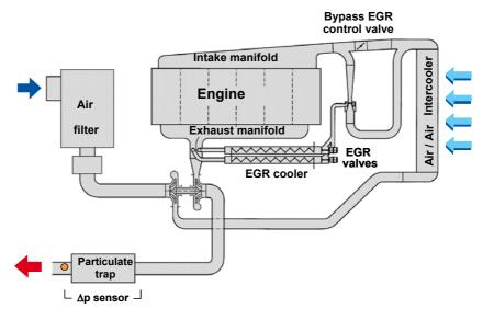
Figure 75: High pressure EGR (Source: AVL)
