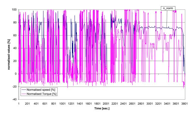
Figure 18: TNO real world test Cycle (7 kW/ton)
