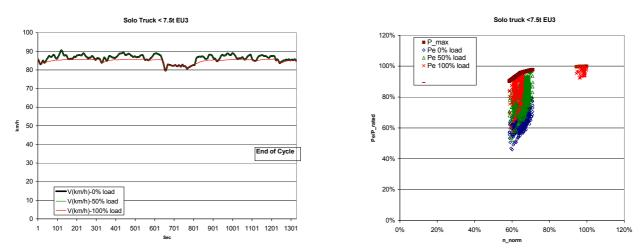
**Figure 86:** Cycle 1020 (Highway standard, 2% gradient) simulated with a solo truck < 7.5t, EURO 3 (cycle= left, engine load = right)
