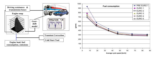
Figure E1: Schema of the model PHEM (left) and simulated fuel consumption values for the HDV-category "semi trailers 34-40t", half loaded, 0% road gradient
