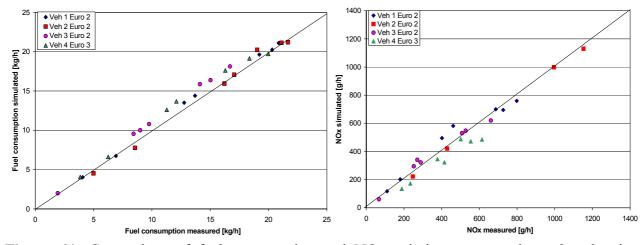
Figure 64: Comparison of fuel consumption and NO<sub>x</sub>-emissions measured on the chassis dynamometer versus the simulated values
