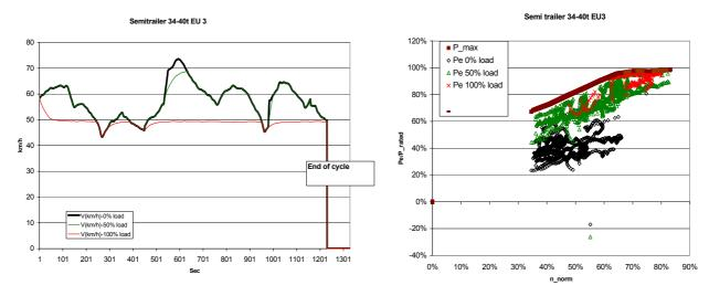
Figure 87: Cycle 1130\_4s\_loaded (Highway standard, 4% gradient) simulated with a semi trailer 34-40t, EURO 3 (cycle= left, engine load = right)
