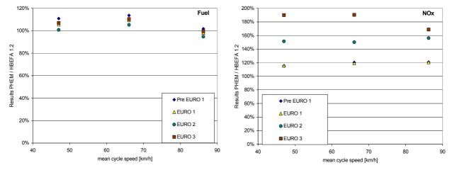
**Figure 98:** Comparison of the fuel consumption and NO<sub>x</sub> emission factors calculated here (model PHEM) with the emission factors from the Handbook Emission Factors (HBEFA 1.2) for three driving cycles with 0% road gradient, 50% loaded solo truck 14-20t
