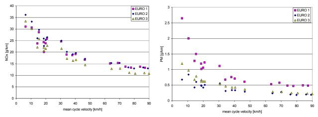
Figure 101: Simulated NOx- and particulate emission factors for truck trailers and semi trailers 34 to 40 tons, 100% loaded, +/-2% road gradient
