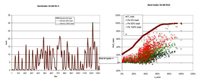
Figure 88: Cycle 13023 (Congested, 6% gradient) simulated with a semi trailer 34-40t, EURO 3 (cycle= left, engine load = right)
