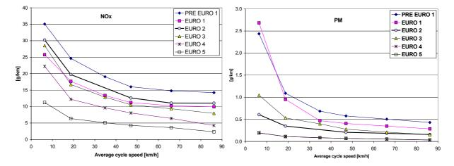
Figure E3: Simulated emission factors for NO<sub>x</sub> and particulate matter for the HDV-category "semi trailers 34-40t", half loaded, 0% road gradient
