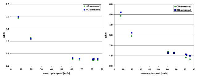
Figure 67: Comparison of the HC- and the CO-emissions measured on the chassis dynamometer versus the simulated values for the average of all measured HDV
