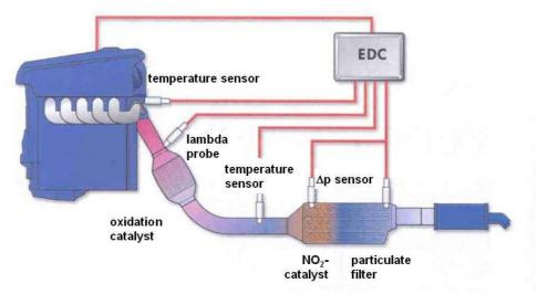
Figure 72: Schematic picture of a continuously Regenerated Filter
