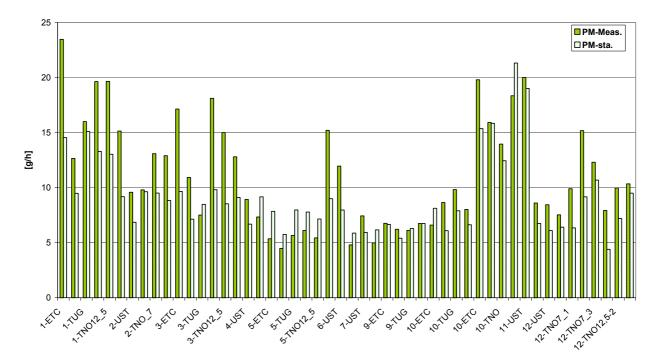
Figure 41: Deviation between the result of the quasi-stationary recalculation of the particulate emissions ("PM-sta.) and the measured emission values for the transient tests of all engines. The numbers give the engine number code (1-ETC means "engine one in the ETC")
