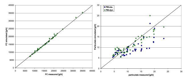
**Figure 44:** Fuel consumption and particle emissions simulated with and without transient correction functions compared to the measured values for all engines in all available transient tests
