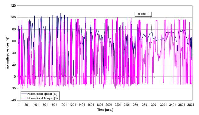
Figure 17: TNO real world test Cycle (12.5 kW/ton)
