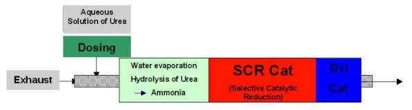
Figure 74: Principle of the SCR Catalyst (Source: PUREM)
