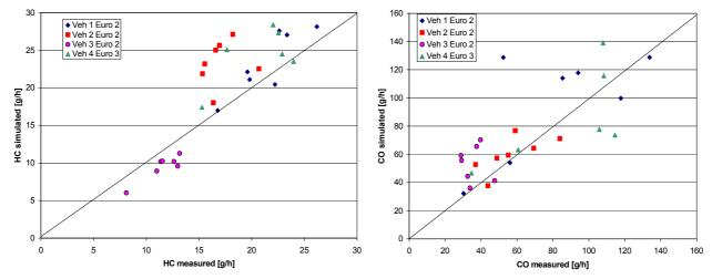
Figure 65: Comparison of HC- and CO-emissions measured on the chassis dynamometer versus the simulated values
