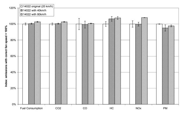
**Figure 60:** Emissions measured for a EURO 2 HDV with different settings of the fan speed in a city cycle (km/h = fan speed)
