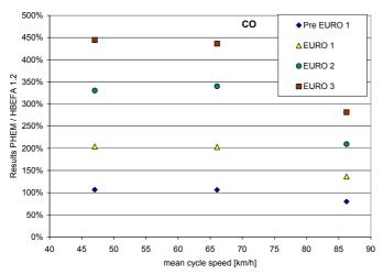
**Figure 100:** Comparison of the CO emission factors calculated here (model PHEM) with the emission factors from the Handbook Emission Factors (HBEFA 1.2) for three driving cycles with 0% road gradient, 50% loaded solo truck 14-20t
