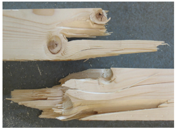
Abb. 5-12: LSF, AA; Zugbeanspruchung
