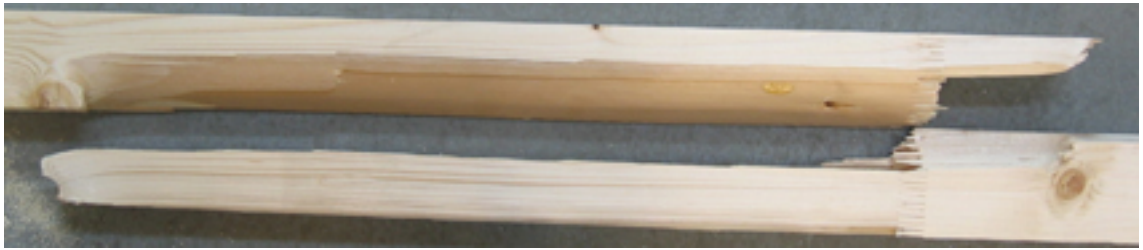
Abb. 5-14: LSF, SSA, RS; Zugbeanspruchung
