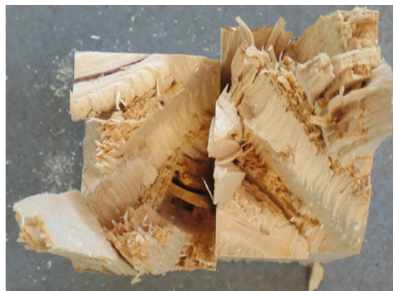
Abb. 5-13: LSF, AA; Zugbeanspruchung
