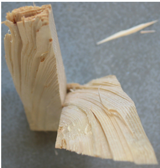
Abb. 5-15: GSF, DW; Zugbeanspruchung
