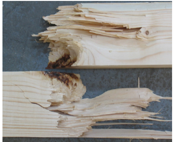
Abb. 5-23: RE, LSF; Zugbeanspruchung
