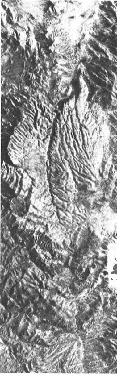
FIGURE 7c Result of a first attempt at combining the LANDSAT data and radar image of Figures 7a and b. (Courtesy of Goodyear Aerospace Corp.)
