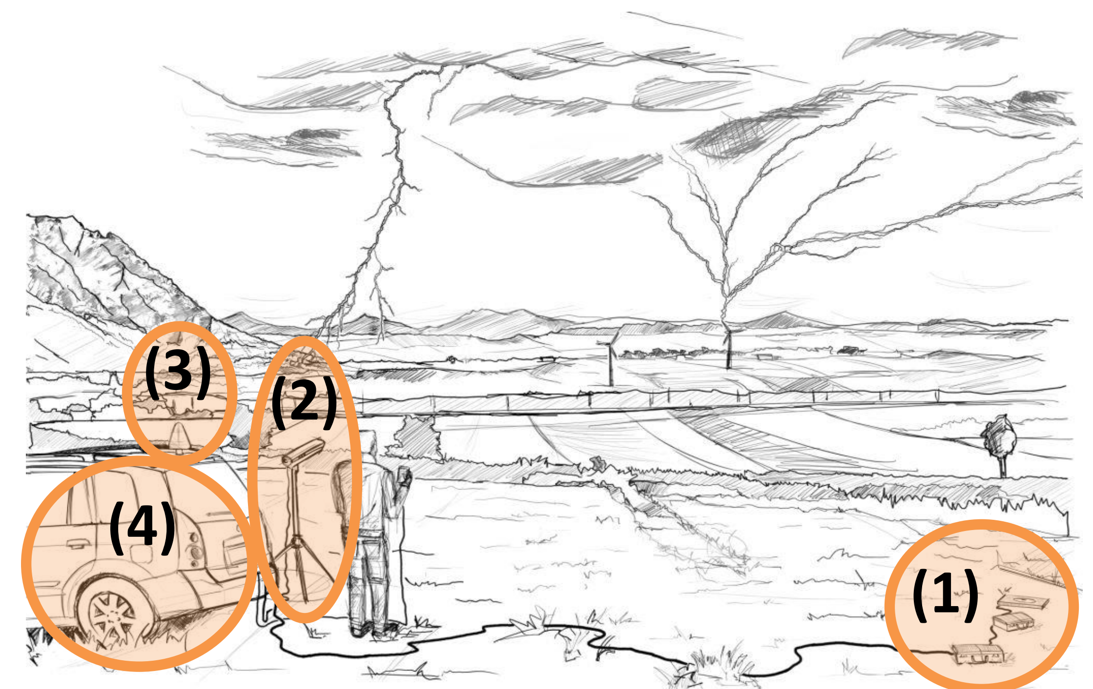
Figure 2: Schematic of the Video and Field Recording System operated in the field: (1) Electric field sensor, (2) Camera, (3) GPS antenna, (4) Car with inside components (e.g. data acquisition)
