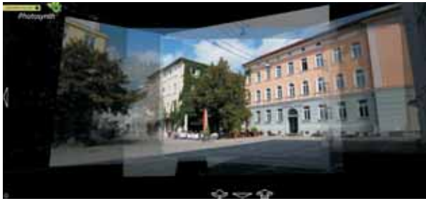
Photosynth Output - The block of images is triangulated, a sparse cloud of 3D points has been computed and the individual photographs can now be navigated in 3D.
