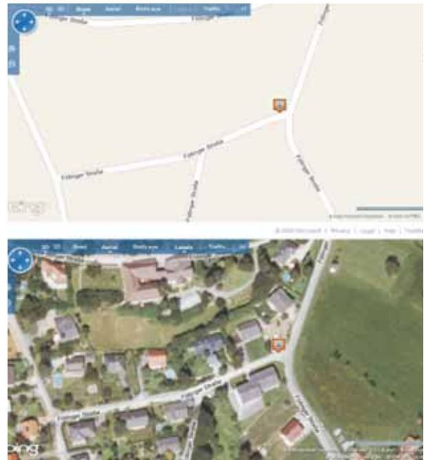
Example of a 2D street map and the vastly enriched information when superimposed by an orthophoto.. This example is being taken from www.bing.com/maps .
