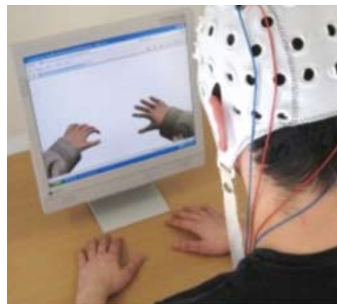
Fig. 3: A BCI user during feedback training. The participant's task is to imagine left- and right-hand movements. The BCI generates opening and closing movements of the left or right (virtual) hand according to classified brain patterns.
