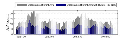
Figure 4.25: Count of different BLE access points throughout the test circuit with roof mounted antennas
