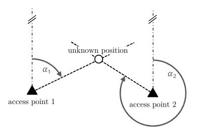
Figure 3.2: Schematic representation of angulation using two access points
