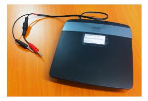
Figure 4.2: Linksys E2500 router with cables for an external, portable power source
