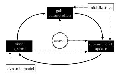
Figure 3.6: Principle of the Kalman filter [17, p. 54]
