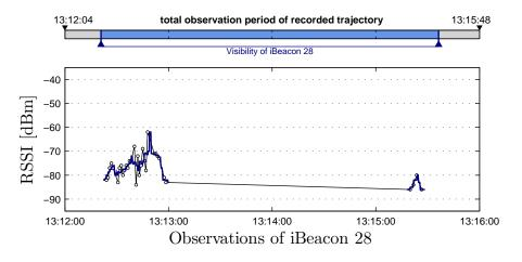
Figure 4.17: Filtered and interpolated observations (1 Hz) from BLE access point 28, showing a circuit through the Thondorf parking deck. Used filter window width is  $\pm 2$  s and interpolation interval is 0.25 s. The computed data is displayed as a blue line.
