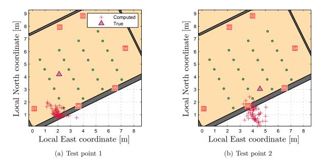
Figure 4.26: WLAN-based lateration in the A111 lecture room, using the EDiMAX dongle. The access points are shown as orange squares, the green circles represent the fingerprinting reference points and do not serve a purpose here.
