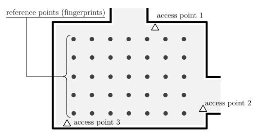
Figure 3.3: Schematic representation of fingerprinting in a building
