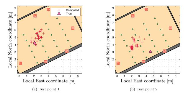
Figure 4.9: Static positioning (60 seconds) on selected test points marked as pink triangles, the used WLAN antenna was the EDiMAX dongle. Positions were computed using a WKNN fingerprinting with K = 4 nearest neighbors.
