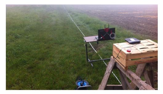
Figure 4.4: Arrangement for determining the relation between distance and RSSI for WLAN signals using a Lenovo Z580 and both WLAN antennas simultaneously. The arrangement for Bluetooth is analogous.
