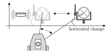
Figure 4.28: Test setup for time synchronization using distinctive observations in both signal domains
