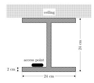
Figure 4.12: Schematic view of the steel girders located at the ceiling of each floor and the placement of an access point
