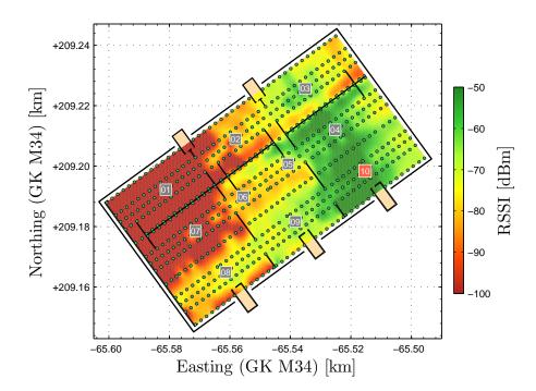
Figure 4.15: Interpolated radio map for WLAN access point 10
