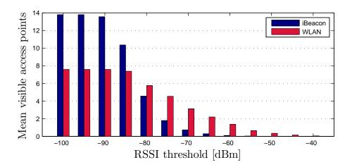
Figure 4.19: Mean number of visible access points per reference point of the radio map representing the Thondorf parking deck under the effect of various RSSI thresholds
