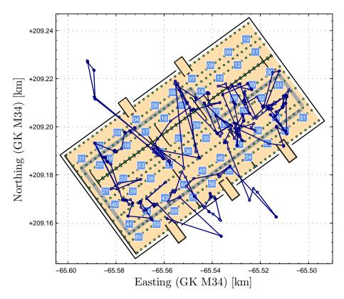
Figure 4.27: Lateration results using BLE data (filtered with a 2 s window, interpolated at 0.25 s and truncated at -85 dBm). The displayed trajectory is a circuit through the parking deck by foot.
