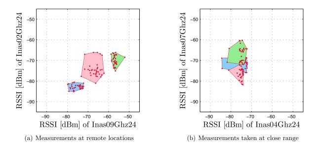
Figure 3.5: 2D feature space showing clustering of measurements from two WLAN access points, showing both an example for easily distinguishable fingerprints and an example for a similar feature representation (caused by a close spatial distance between fingerprints)
