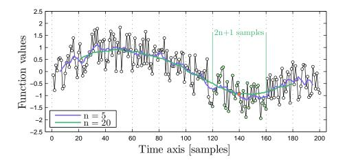
Figure 4.16: Example for two different moving average filters applied onto a noiseaffected sine oscillation. The filter window for t = 140 (red dot) is visualized for a width of n = 20 (2n + 1 samples total).
