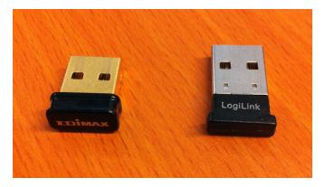
(a) EDiMAX (WLAN) and LogiLink (BLE) antennas
