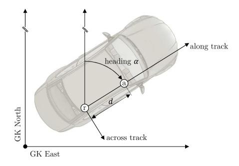
Figure 4.32: Relationship between the geodetic coordinate system and the car system
