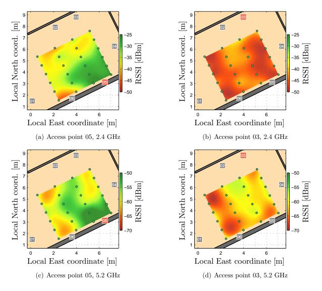
**Figure 4.8:** Radio map visualization by interpolation of RSSI for selected access points. For the displayed examples, the used WLAN antenna was the CSL product.
