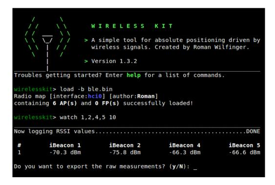
Figure 4.3: Sample screenshot of *Wireless Kit*. First, an existing binary file with previously saved access points is loaded using the command load, then using the command watch some of those access points are observed for a total of ten seconds.
