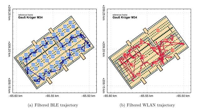
**Figure 4.23:** Computed trajectory resulting from fingerprinting with preprocessed BLE and WLAN measurements. Observations were taken inside a car, with a sampling rate of approximately 1 Hz. The preprocessing parameters are listed in Table 4.4.
