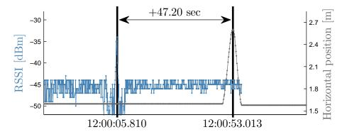
Figure 4.29: Results for time synchronization setup using distinctive observations in both signal domains
