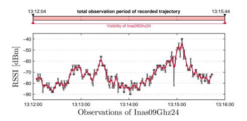
Figure 4.18: Filtered and interpolated observations from WLAN access point 09, showing a circuit through the Thondorf parking deck. Used filter window width is  $\pm 2$  s and interpolation interval is 0.25 s. The computed data is displayed as a red line.
