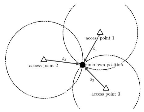
Figure 3.1: Schematic representation of lateration in 2D space
