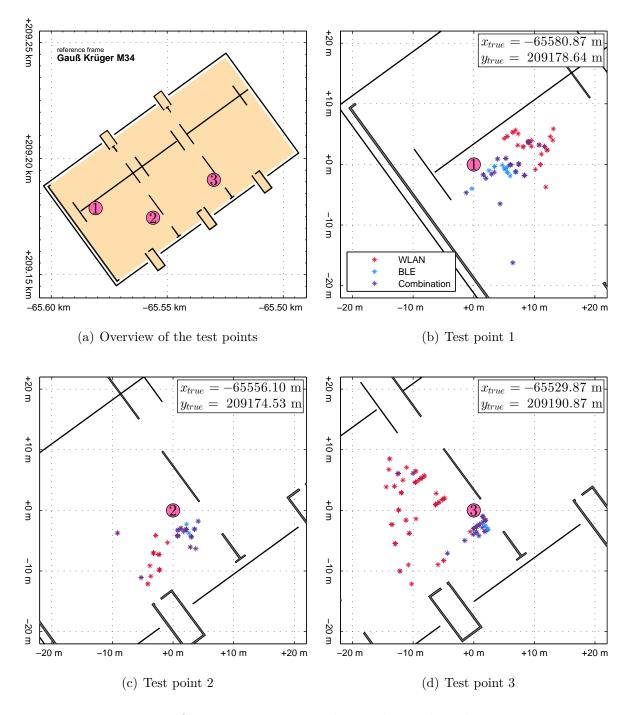
Figure 5.1: Static positioning results on three selected test points
