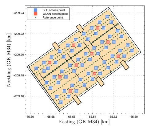
Figure 4.13: Overview of the radio map established on the 5<sup>th</sup> floor of the Thondorf parking deck in December 2014. The access points are placed along steel girders that run across the ceiling of each floor, e.g., the BLE access points 10, 11, 30, 31, 50 and 51 are placed on the same beam. The used coordinate system is Gauß-Krüger M34.
