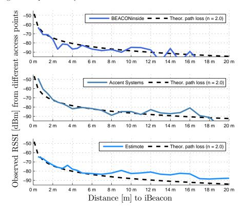
**Figure 4.6:** Empirically determined relation between distance to different BLE beacons and observed RSSI in comparison with the theoretical path loss.
