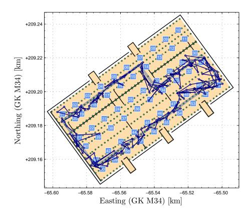
Figure 4.20: Computed trajectory resulting from fingerprinting with raw BLE measurements. Observations were taken by foot, with a sampling rate of approx. 1 Hz.
