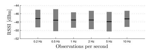
Figure 2.4: Signal strength and standard deviation for various advertising intervals of static observations for a total of 1 min each. The mean signal strength is drawn in black, the corresponding standard deviation as gray bars.
