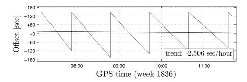
Figure 4.31: Time offset of the Asus Eee PC relative to the GPS time
