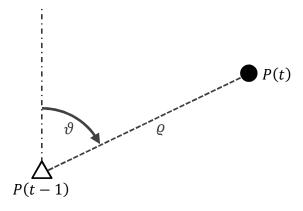
Figure 3.4: Schematic representation of dead reckoning using distance  $\rho$  and angle  $\vartheta$
