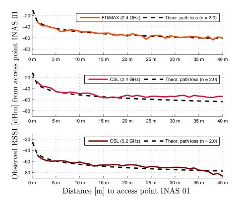
Figure 4.5: Empirically determined relation between distance to access point INAS 01 and observed RSSI in comparison with the theoretical path loss for both investigated WLAN devices.
