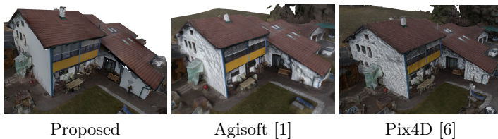
Fig. 3. Results from commercial reconstruction pipelines of the House dataset compared with the proposed approach. Compared to the reconstruction of the proposed approach, Agisoft and Pix4D do not generate planar surfaces and straight edges, as they use no shape or semantic priors. The facades and roofs are noisy and scene are smoothed too much and become rounded (e.g., building edges, chimney).
