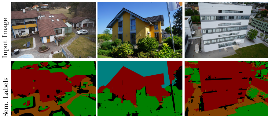
Fig. 4. Semantically labeled input images from the House (left), Residential Area (middle) and Block Building (right) datasets. The pixels are labeled as sky (blue), building (red), vegetation (green), road/pavement (brown) and clutter (black). The labeling is not always perfectly correct. However, due to the redundancy, the 3D points have less errors in labeling (see Fig. 5).
