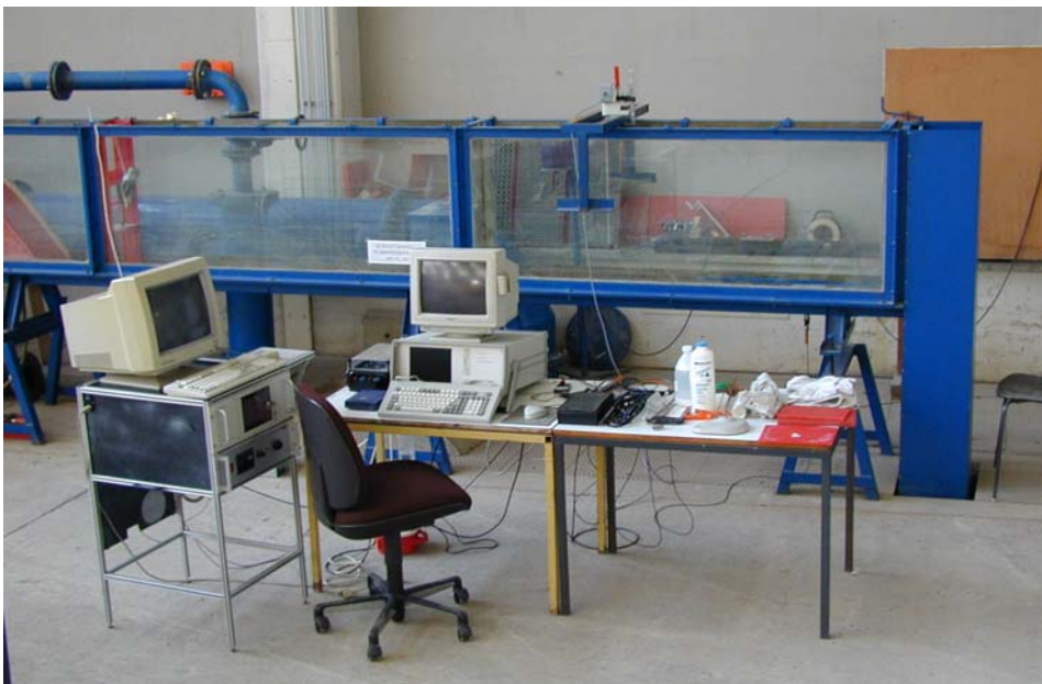
Figure 5-2: Test facilities for employing the UVP-Monitor in the study of open channel flow.
