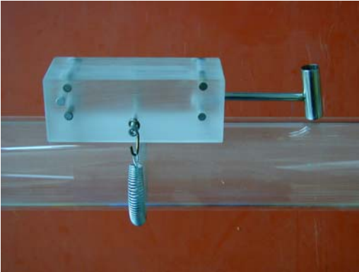
Figure 4-5: Support for fixing the transducer on the pipes.
