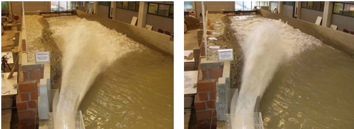
Figure 13. Flip bucket for a full reservoir ( T.W.L. 625m above datum) and 100% gate opening; left: initial condition, right: Variant 1
