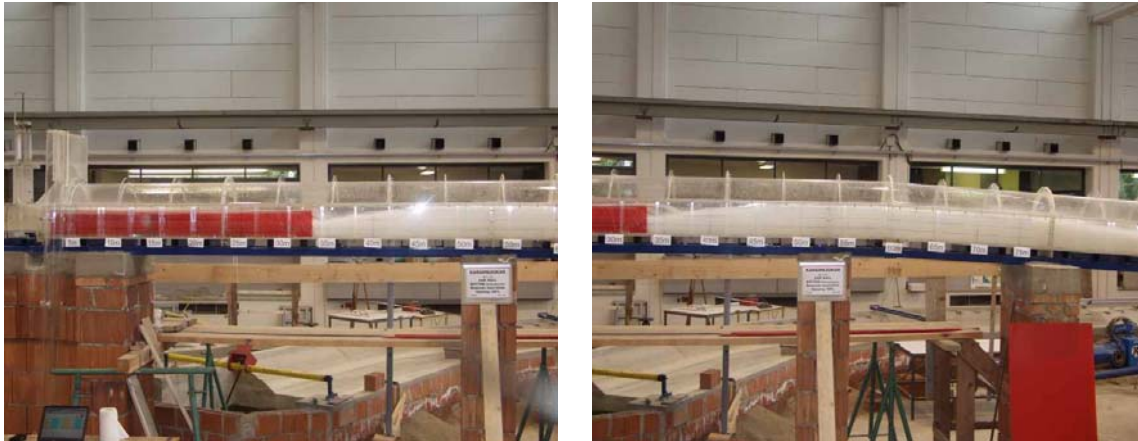
Figure 9: Flow behaviour for vertical baffles with invert remaining at the initial level, for a full reservoir (T.W.L. 625m above datum) and 100% gate opening (= final proposal)
