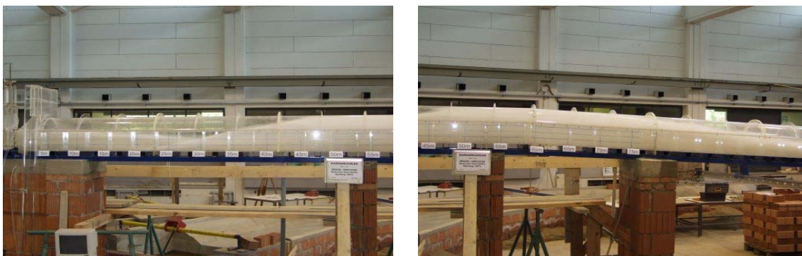
Figure 8. Rooster-tail development for a full reservoir (T.W.L. 625m above datum) and 100% gate opening, in the initial condition
