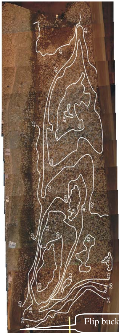
Figure 15: Scour pattern developing after operating flip bucket Variant 2 for a major length of time
