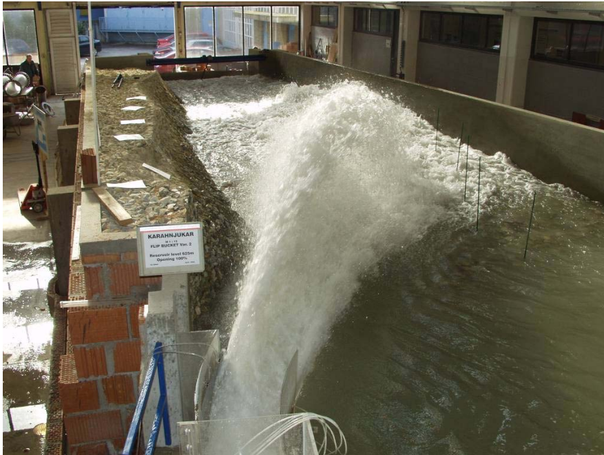
Figure 14. Flip bucket for a full reservoir ( T.W.L. 625m above datum) and 100% gate opening – final proposal (Variant 2)
