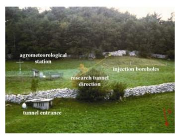
FIG. 3. Surface installations at the RS Sinji Vrh — agrometeorological station, injection borehole for multi-tracer tests and area where fertiliser was applied.
