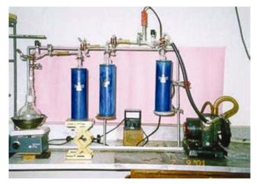
FIG. 3. Soil moisture extraction system.
