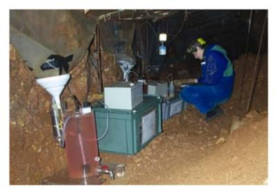
FIG. 5. Construction for collecting water samples in the tunnel with automatic device for flow rate and fluorometer for the multitracer experiment.
