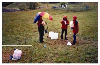
FIG. 13. Injection of the tracer 'cocktail'..
