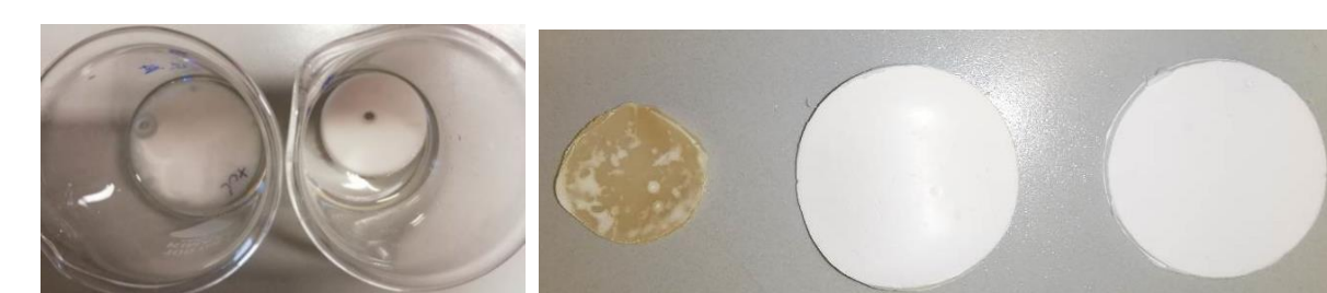
Photographs of specimens during and after swelling procedure in toluene.
