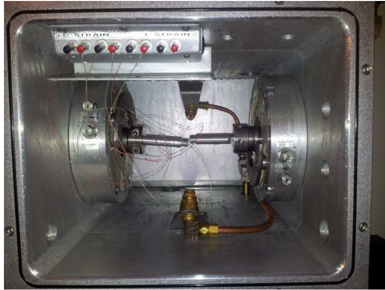
Figure 2: A broken hot torsion specimen after quenching in the Gleeble® 3800. For temperature measurement and heat control, thermo-couples were mounted in the middle and edge of the twisted area.
