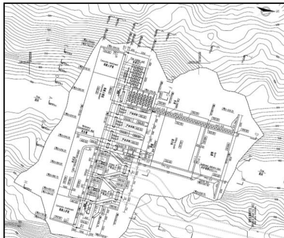
Figure 2. Regulating Dam HEPP Poso-I Lay out
