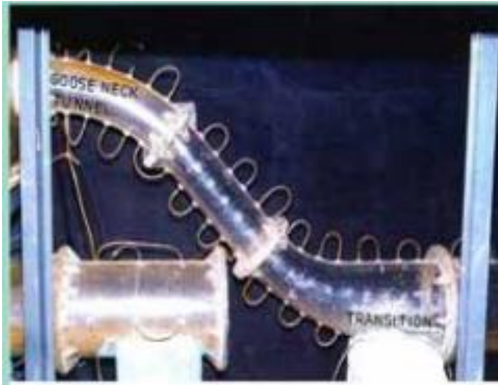
Figure 2 Photograph of the model showing diversion and depletion tunnels
