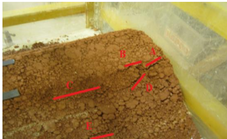
Figure 13: Upstream damage after reservoir with vibration at resonance condition
