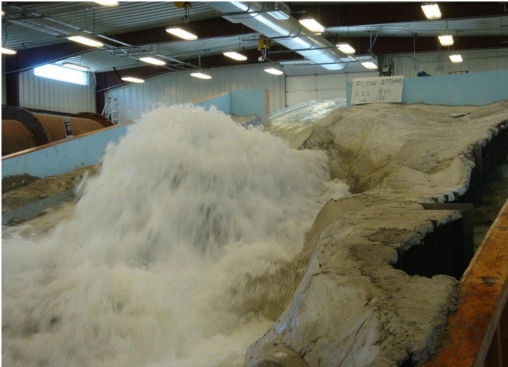
Fig. 6 Performance of plunge pool alternative of Oroville Dam's FCO Spillway chute
