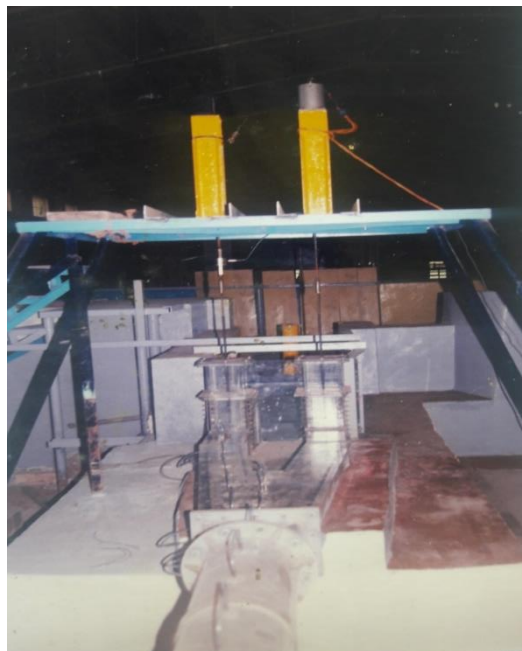
Figure-3. Typical Set Up For Estimation of Hydrodynamic Forces on Service Gate
