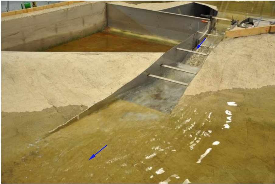
Figure 8. Energy dissipation at 475 m 3 /s from the new spillway, with the existing spillway in the closed position.
