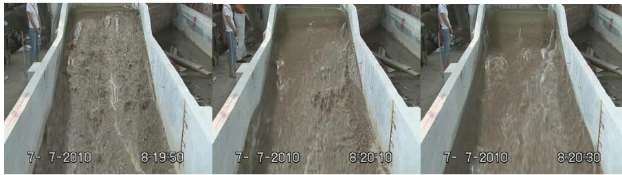
Figure 7 Test photo of entire Overtopping dam erosion
