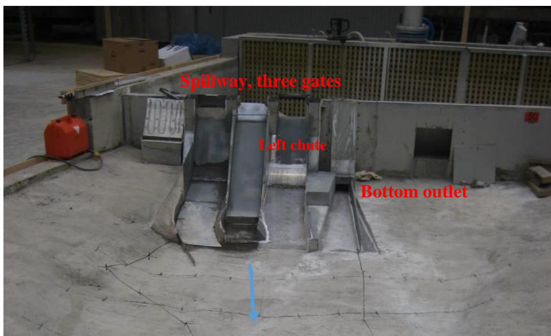
Figure 11: Hydraulic model of Ramsele dam, scale 1:50, with the proposed prolonged left chute (Vattenfall R&D, 2014)
