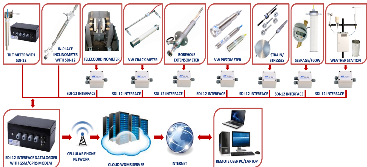
Fig. 5 Dam monitoring instruments on an SDI-12 network
