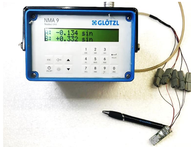
Fig. 13. Glötzl hand-held readout unit for inclination sensors connected to the MEMS
