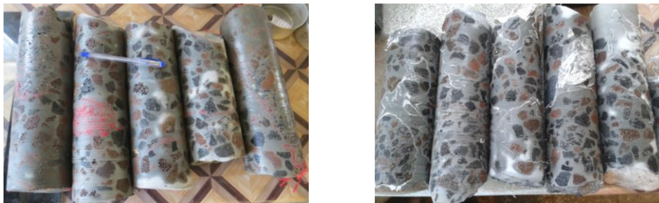
Fig. 3 Left: Core of Onion Sacks, Right: Core of Flour Sacks
