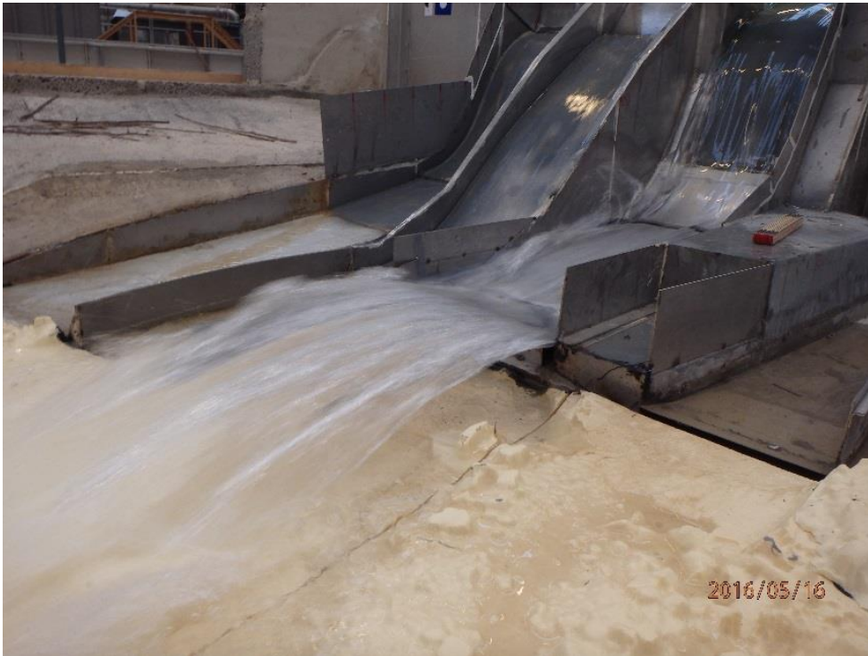
Figure 12: Ramsele, left spillway – proposed shortened ski jump design (Norconsult, 2016)
