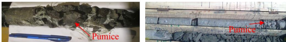
A: Core sample of ISA panel B: Core sample of FLA panel
