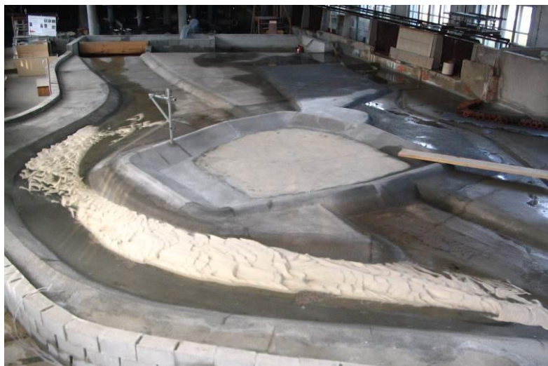
Fig. 5: Physical model of the HPP Brežice construction pit (Hidroinštitut, 2011). In the diversion channel the remains of the sand left from studying sediment transport capacity are evident
