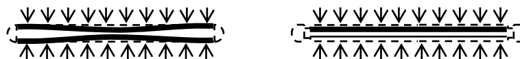
Fig. 5. Deformation of welded edge and grooved edge pressure cushions under uniform pressure in fine soil materials
