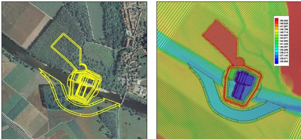
Fig. 4: Left – an orthophoto image with the developments in the HPP Brežice construction pit site; right – the same site captured using the numerical mesh of the 2D hydraulic model [4]
