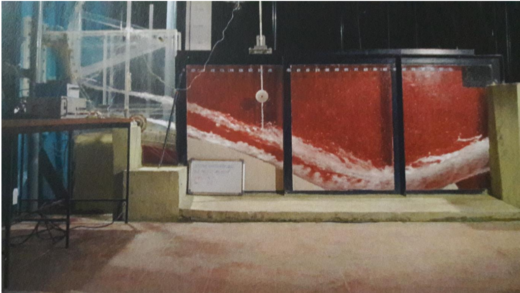
Figure1. Model set up for measurement of air concentration in an orifice spillway overflow
