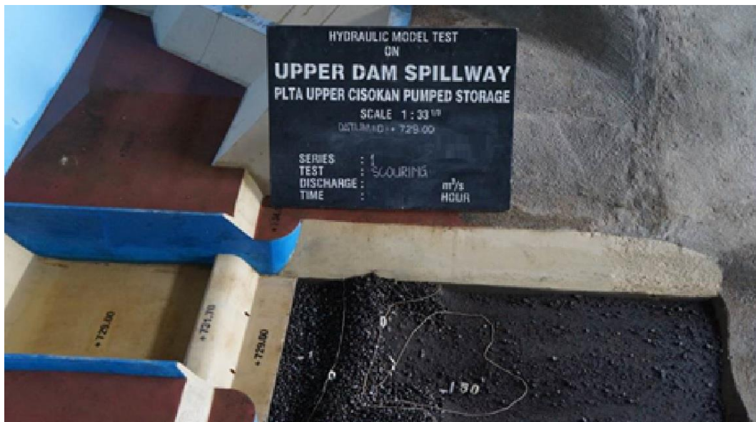
Fig. 11. Scouring condition at downstream of spillway (Scenario 2)
