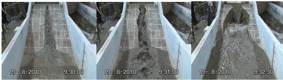
Figure 9 Test photo of headcut erosion
