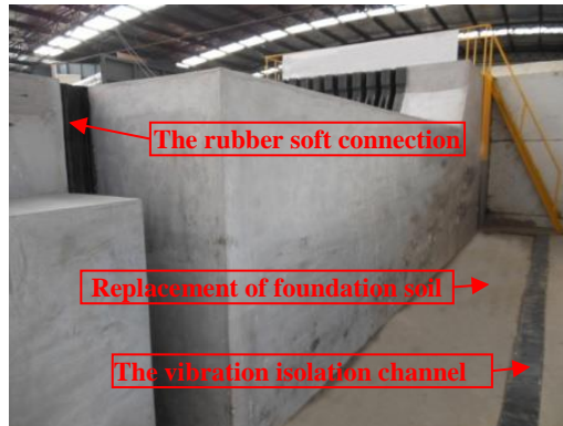
Fig. 4 Vibration isolation and reduction measures of the model
