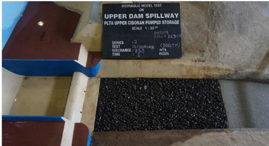
Fig. 12. Scouring condition at downstream of spillway (Scenario 3)
