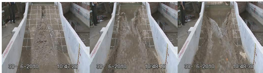
Figure 5 Test photo of layer-by-layer dam erosion
