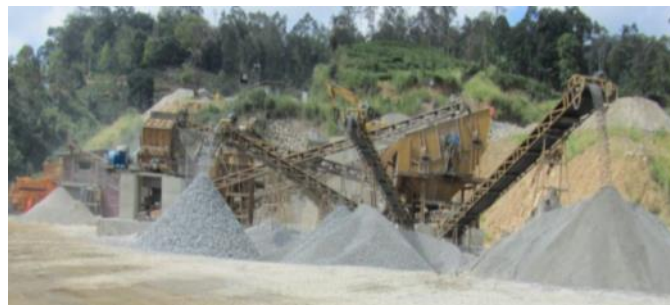
Fig. 1 Aggregate production in stone crusher (Uma Oya project-Sri Lanka)
