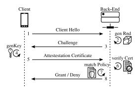
Figure 4: Initial connection between client and back-end.
