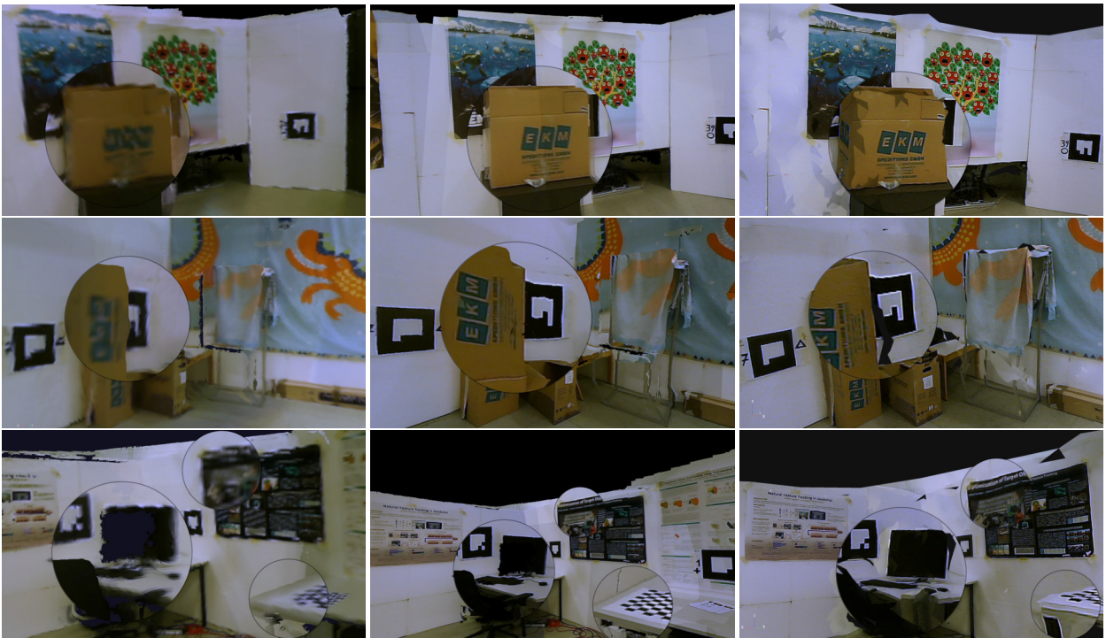
Fig. 15. Comparison of our method to per-vertex colored KinectFusion model and to an offline-reconstruction rendering using a leading commercial photogrammetry (3DF Zephyr). From left to right: (a) KinectFusion's rendering (b) our rendering (c) 3DF Zephyr's rendering results.
