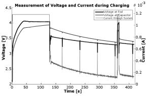
Figure 4: Measurement of the charging of prototype A.
