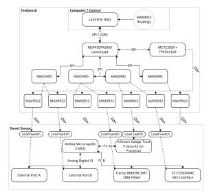
Figure 2: Design of prototype B.
