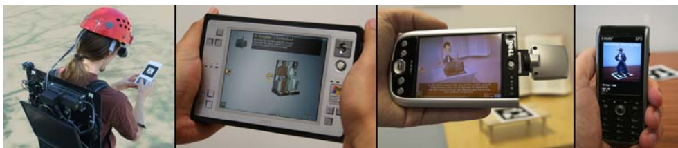
Abb. 2: Evolution von Augmented Reality Systemen: „Backpack“-AR System, Ultra-Mobile PC, PDA, Smart Phone (vlnr).
