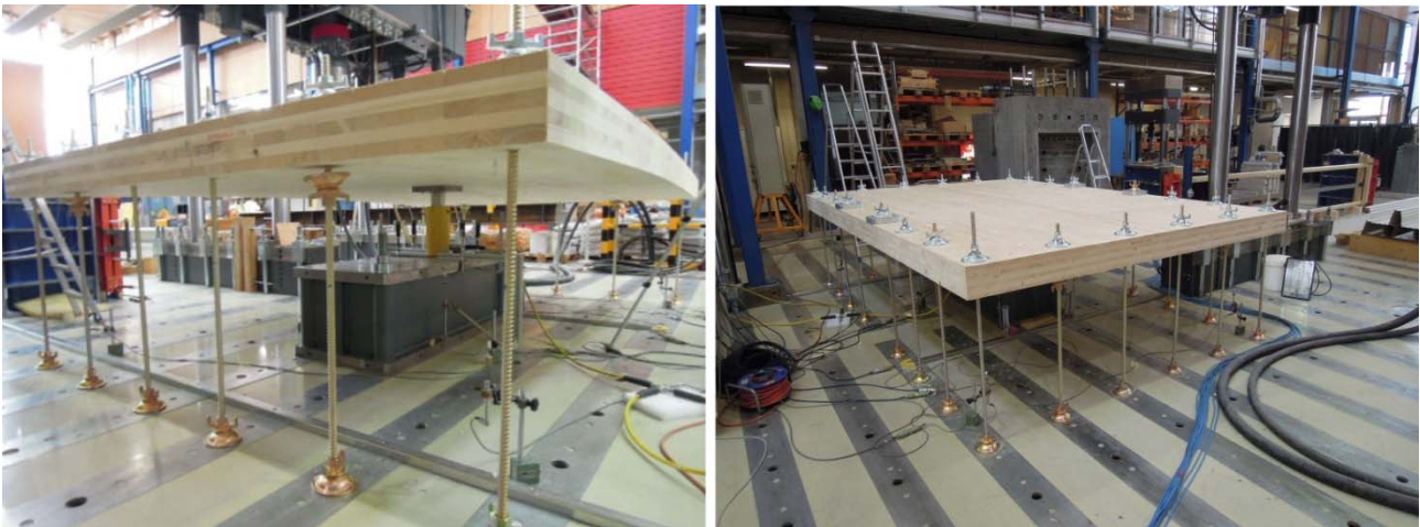
Figure 4.5. Images of test configuration 2 for test series with expected bending failure mode
