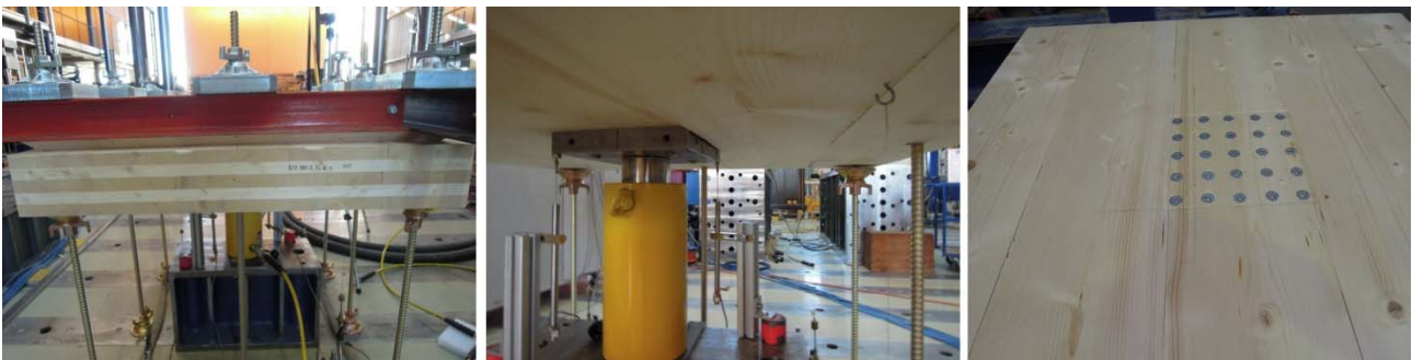
Figure 4.3. Images of test configuration for expected punching shear failure (test configuration 1)
