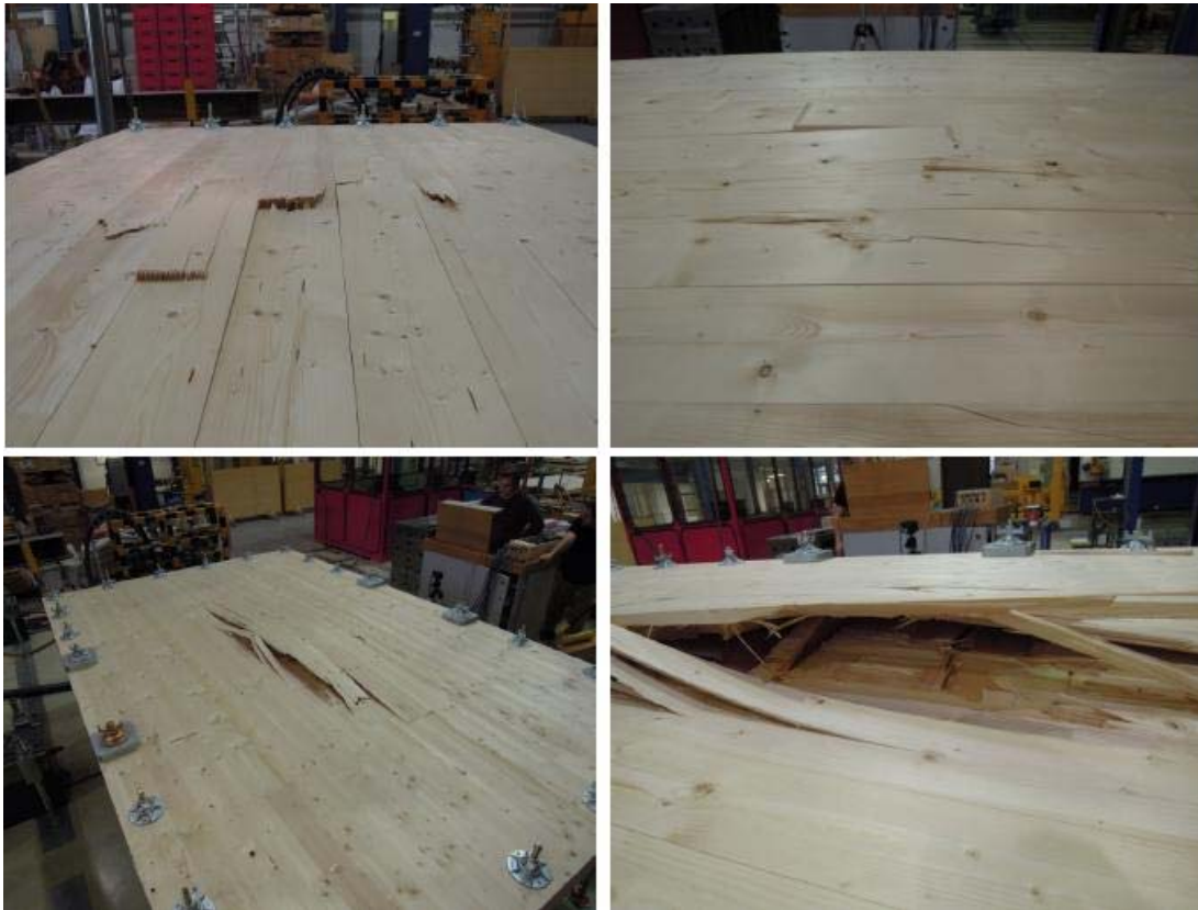
Figure 5.3. observed typical failures in test configuration 2
