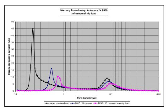
Figure 5 Series 3: The influence of nip load on pore structure
