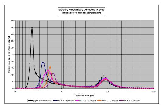
Figure 3 Series 1: The influence of calendering temperature on pore structure
