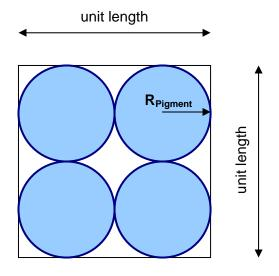
Figure 2 Particle packing of spherical pigments
