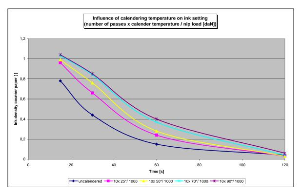
**Figure 8** Ink setting as a function of steel roll temperature at calendering
