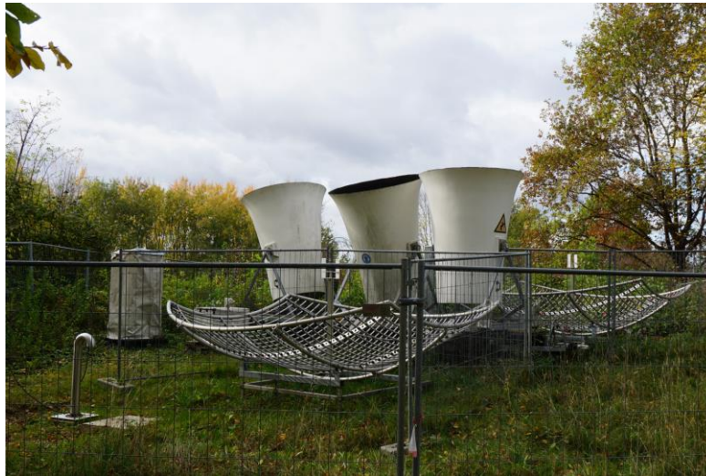
Figure 2. Radio-Acoustic Sounding System (RASS) which is installed at the campus of the University of Augsburg about 300 m north of the ceilometer.
