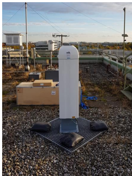
Figure 1. Ceilometers Vaisala CL51 at the roof of the Building of the Institute of Geography of the University of Augsburg.
