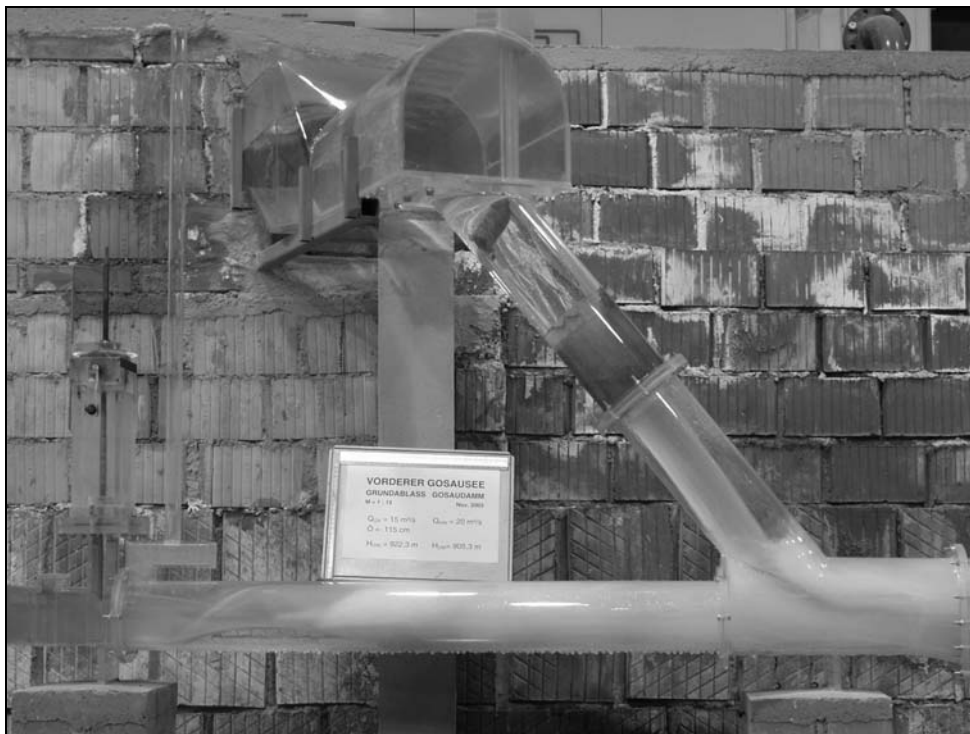
Figure 10. Simultaneous Operation of Bottom Outlet and Spillway ( Q_{BO} = 15 \text{ m}^3/\text{s} , Q_{SP} = 20 \text{ m}^3/\text{s} )
