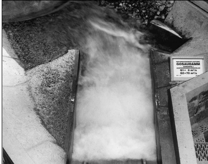
Figure 5. Stilling-basin Alternative ( Q_1 = 70 \text{ m}^3/\text{s} , Q_2 = 0 \text{ m}^3/\text{s} )
